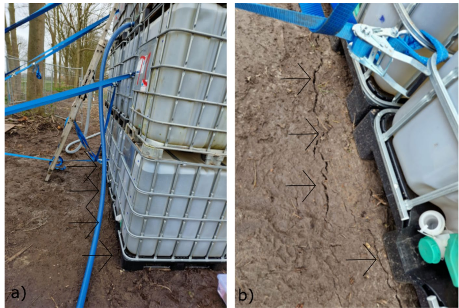
Fig. 9 Initiation of cracks a Cracks running full length behind loading, b Close up view of cracks
