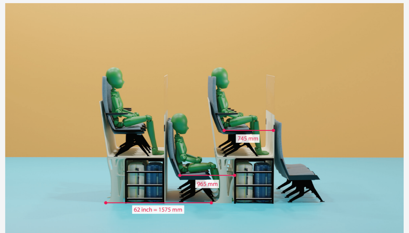
Figure 54 - Mannequins sitting in the final concept, with dimensions of the pitch and legspace.
