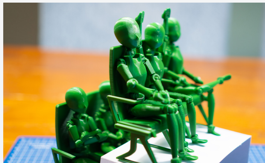
Figure 49 - 3D printed mannequins on the Aero seat in a double decker configuration
