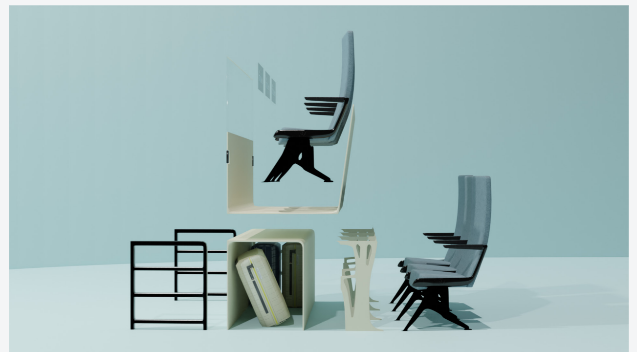
Figure 61 - Above: The double decker seat in the back of the Flying-V. Figure 62 - Below: An exploded view of the main parts of the double decker seat.
