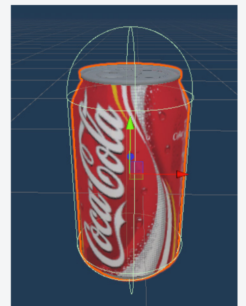
Figure 41 - The collider is visualised with the green lines surrounding the cola Can.
