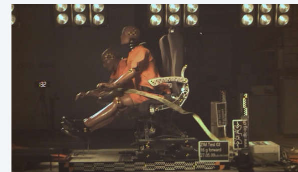
Figure 92 - Screenshot of "Aircraft seat 16 g structural test with ground deformation" - Youtube Channel: DynamicTestCenter
