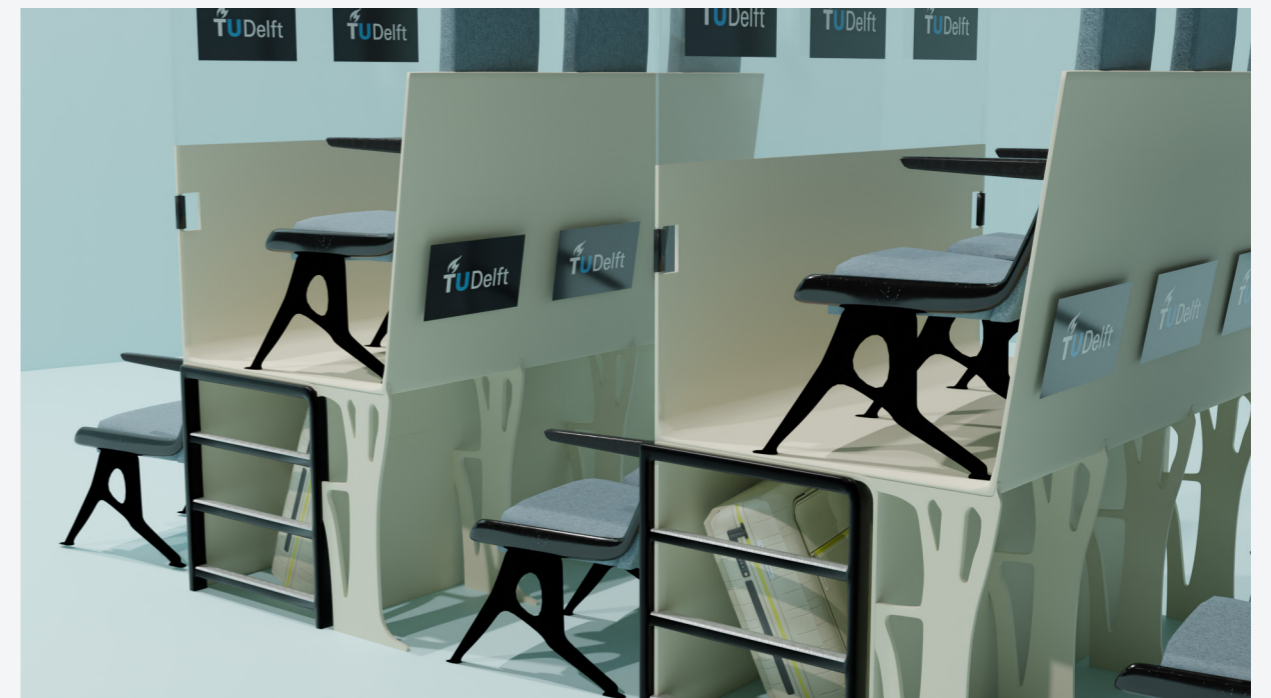
Figure 58 - Picture above shows a sideview of the double decker seat, one luggage fence has been opened. Figure 59 - Picture below shows the double decker seat in more detail.
