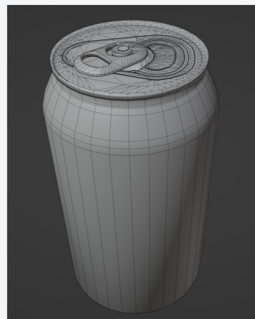
Figure 17 - Add more detail to get can characteristics. The mesh gets more complicated
