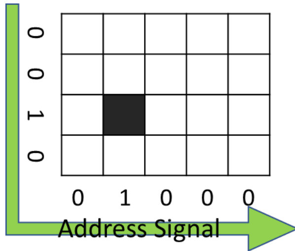
Figure 3.20: Schematic of the Address Selection Process in Piezoresistive Sensor
