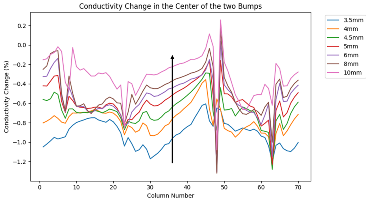
Figure 4.16: The change of conductivity change value at rows 15 and 16 of the differential stress distribution pattern in high bending, the arrow shows the direction of increased bending stress
