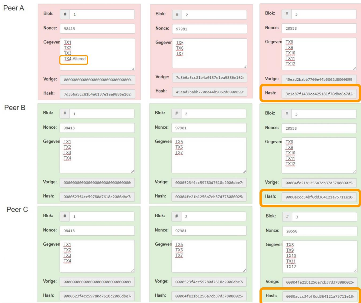
Figure III.11 Display of the impact of altering one transaction in a blockchain consisting of multiple peers (Brownworth, 2020)
