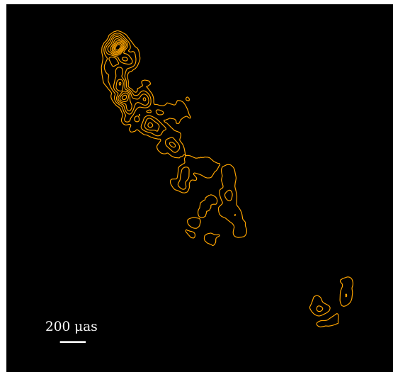
Fig. A.1. CLEAN model in contours of 3C 279 RadioAstron 2018 observations using Difmap and plotted using a Python script. Contours are plotted at levels of 0.1 to 0.9 times the peak brightness, in steps of 0.1.
