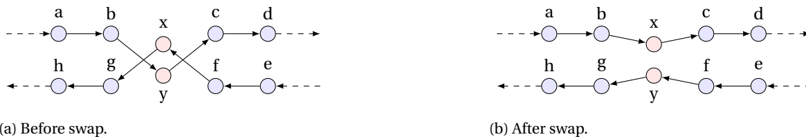
Figure 2.7: Swapping nodes x and y . The node strings can be from the same route or from two different routes.
