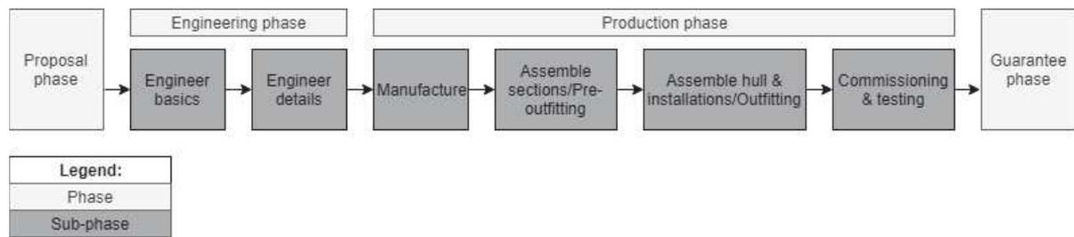
Figure 2.1: Flowchart of the shipbuilding phases and sub-phases at IHC
