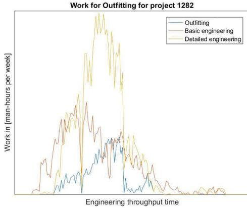
Figure 7.20: Work timing for Outfitting
