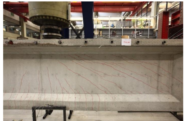
Fig. 14 Crack development beam type 201 (first test)
