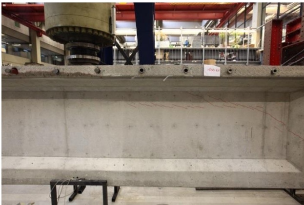
Fig. 14 Crack development beam type 201 (first test)
