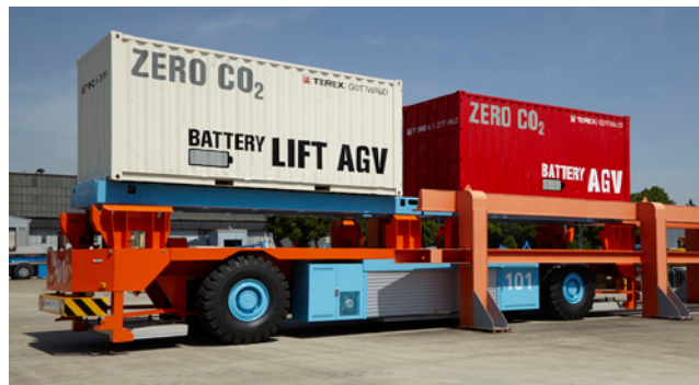
Figure 8: A lift-AGV delivering/collecting containers at a rack (source:www.terex.com).
