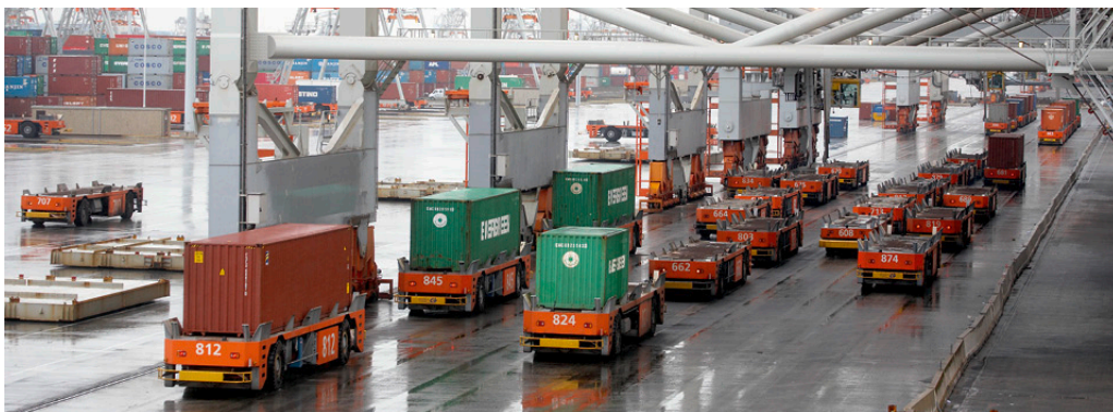
Figure 19: Dispatched AGVs driving towards their task (source: www.demagcranes.fr )
