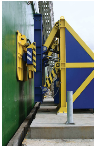
Figure 23: Equipment used to automate the mooring process of a vessel (source: [71])
