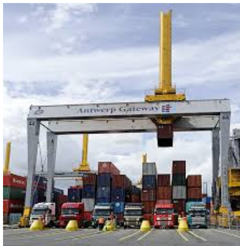
Figure 25: An ASC equipped with a beam in order to counteract sway [source: www.terex.com ].
