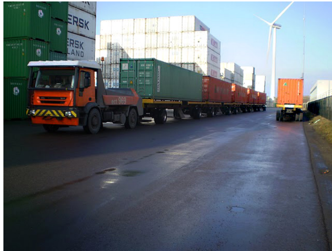
Figure 13: Example of an MTS system at the ECT terminal (source:www.brandigg.de).
