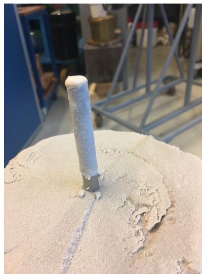
(b) Injection nozzle with external sandscreen
