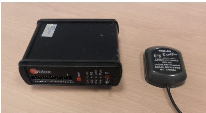
Fig. 2. The u-blox TIM LP single frequency receiver evaluation kit (left) and Tri-M Big Brother patch antenna (right) that were used during the car tests. This hardware is representative of mass-market GNSS hardware for automotive applications.
