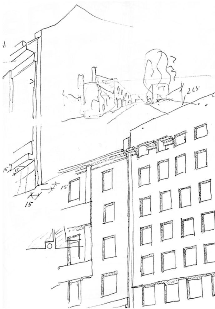
**Figure 5.51.** Álvaro Siza – Sketches for the housing block in Schelesisches Straße. October 1981. Connection of the new construction with the adjacent old building. Source: *Alvaro Siza, City Sketches / Stadtskizzen / Desenhos Urbanos*, ed. Brigitte Fleck, 1st ed. (Birkhäuser, 1994), 75.
