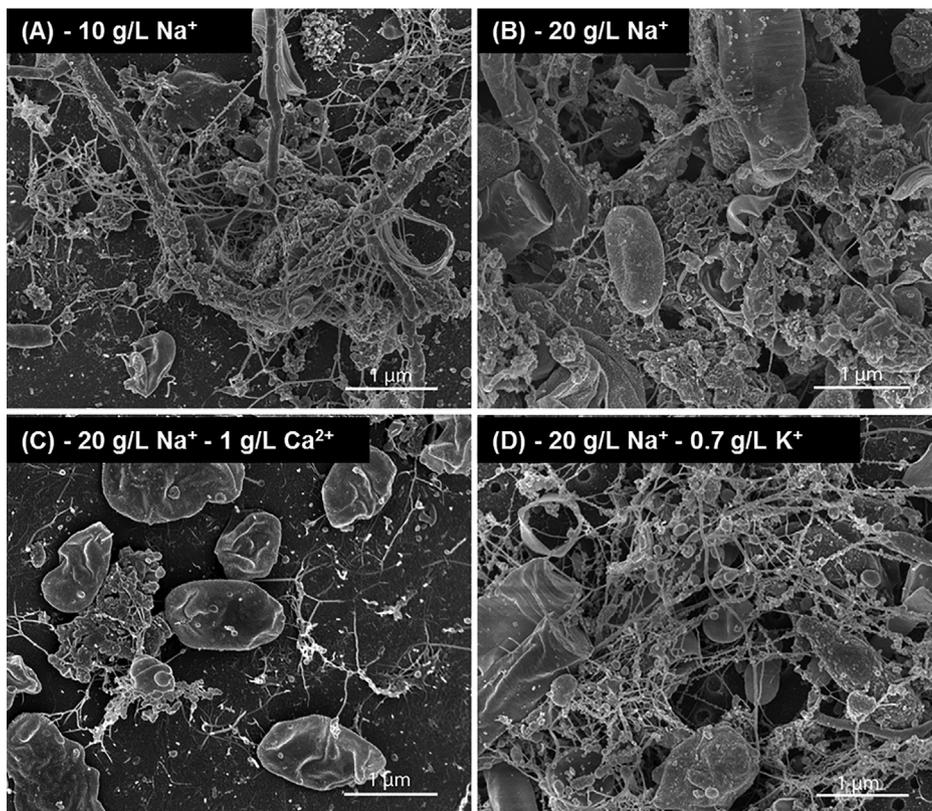
Fig. 3. SEM images of biofilms samples from the reactors B1 (a), B2 (b) B3 (c) and B4 (d) after 40 days of operation.
