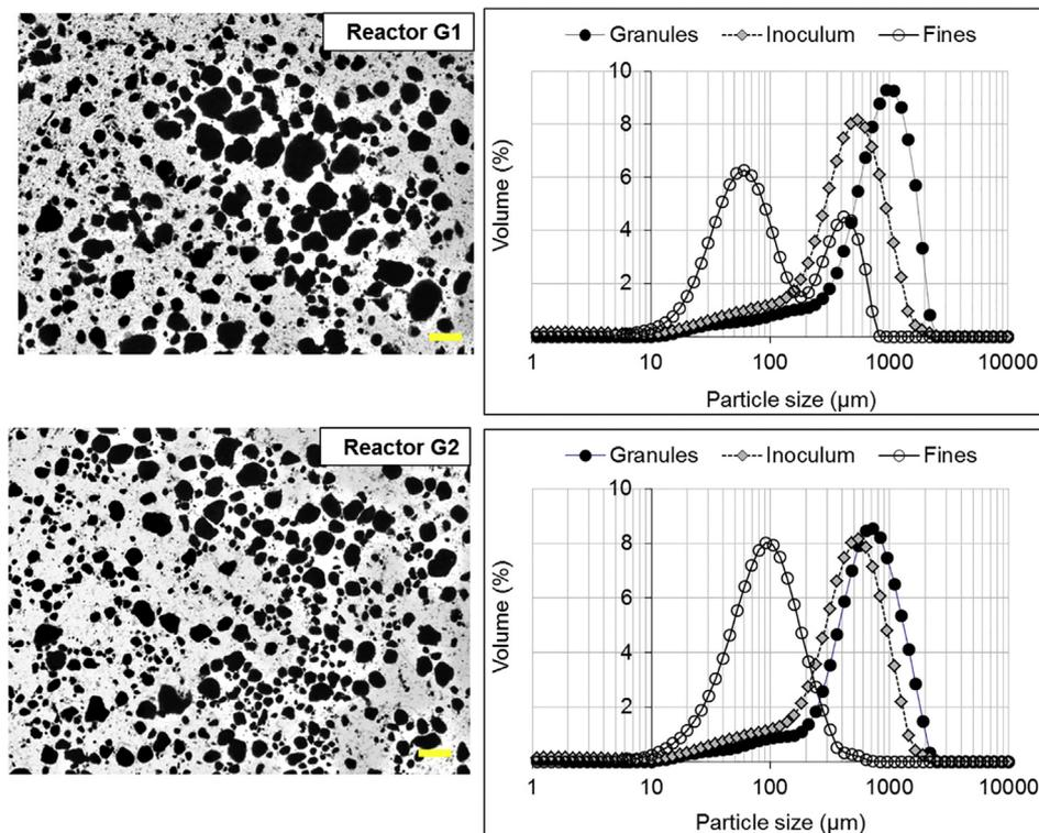
**Fig. 6.** Microscopic images and particle size distribution of sludge from the two UASB reactors as well as for the fines produced in these reactors. Samples were taken after 120 days. Yellow bars in microscopic images are 500  $\mu\text{m}$ . (For interpretation of the references to colour in this figure legend, the reader is referred to the web version of this article.)
