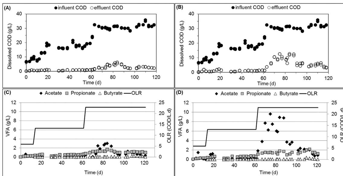
**Fig. 5.** Influent and effluent dissolved COD concentrations, and VFA concentrations for reactor G1 without additional calcium (A and C) and for reactor G2 with additional calcium (B and D).
