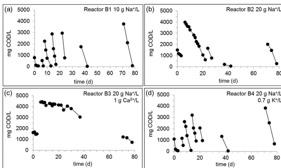
**Fig. 2.** - Acetate-COD concentrations in reactors B1 (a), B2 (b) B3 (c) and B4 (d).
