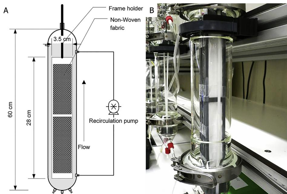
Fig. 1. Schematic representation (A) and picture (B) of an up-flow fixed-bed column reactor used to evaluate microbial adhesion on fixed materials.
