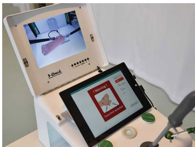
Fig. 4 Instant force feedback system shown on tablet
