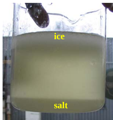
Figure 8.9: Gravitational separation of ice and salt crystals formed by EFC
