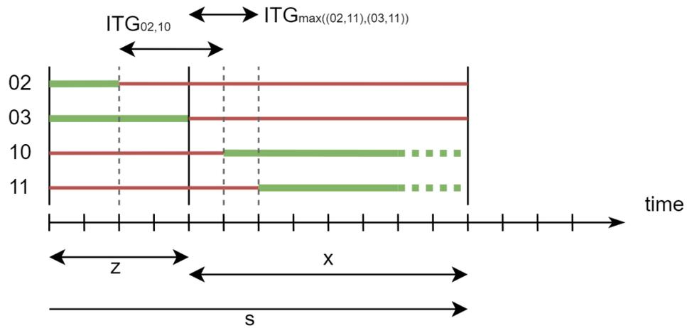
Figure 3.12: A premature ending of green of signal group 02 allows signal group 10 to realise two time intervals earlier. See the caption of Figure 3.11 for further details.
