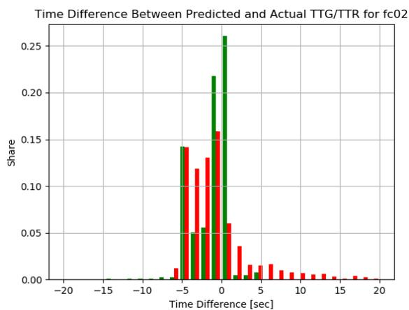
Figure E.38: The TTG and TTR accuracy distribution for signal group 02 in scenario 8 (major-minor, vehicle arrivals).
