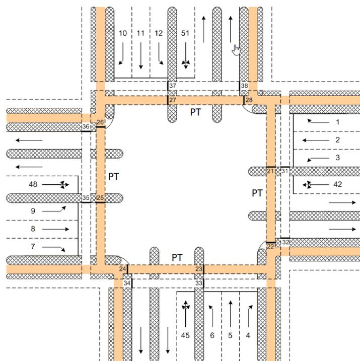
Figure A.1: Dutch coding for signal groups applied to a typical four-leg intersection. The abbreviation of PT relates to public transport (figure source: Wegenwiki, 2015).
