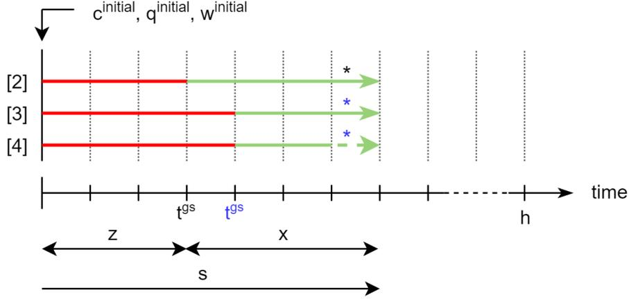
Figure 3.16: Visual representation of the time intervals  $k$  over which the delay is calculated for any signal group  $\lambda$  that may become green within the limited horizon  $s$ .
