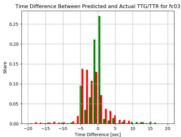
Figure E.39: The TTG and TTR accuracy distribution for signal group 03 in scenario 8 (major-minor, vehicle arrivals).
