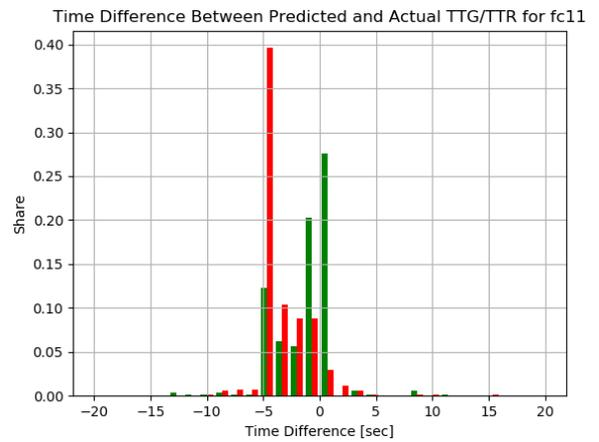
Figure E.46: The TTG and TTR accuracy distribution for signal group 11 in scenario 8 (major-minor, vehicle arrivals).
