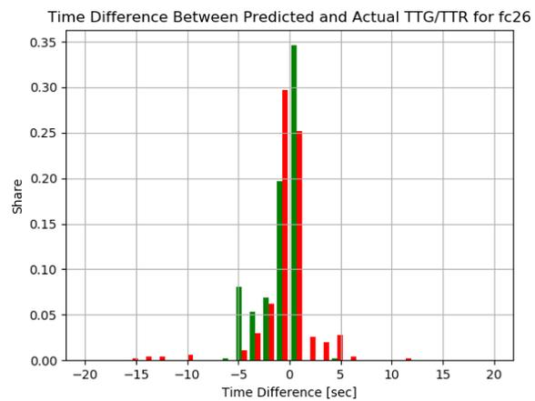
Figure E.48: The TTG and TTR accuracy distribution for signal group 26 in scenario 8 (major-minor, vehicle arrivals).
