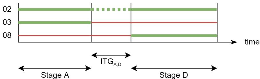
Figure 3.4: An example of a planning of green intervals for signal groups according to a stage-based approach.  $ITG_{A,D}$  denotes the intergreen time between stages A and D. The green time of signal group 02 is cosmetically lengthened over the intergreen interval between stages A and D.
