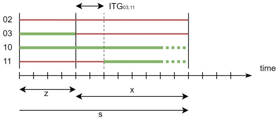
Figure 3.13: The absence of a green request for signal group 02 allows signal group 10 to become green earlier than the start of  $x$ . See the caption of Figure 3.11 for further details.
