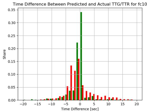
Figure E.33: The TTG and TTR accuracy distribution for signal group 10 in scenario 7 (equal flows, vehicle arrivals).
