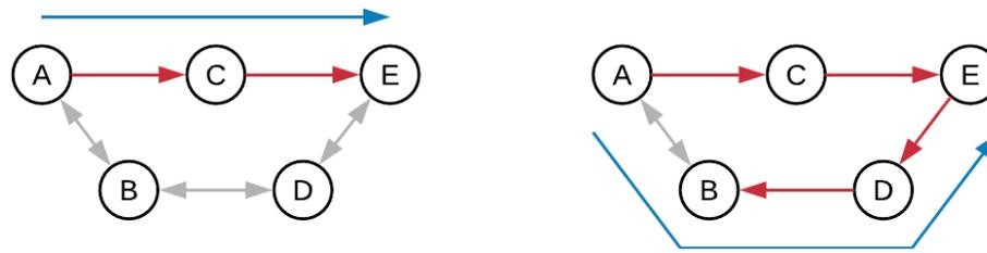
Figure 2.5: A fictional network for a shortest and longest path problem. The blue arrow in the left figure represents the shortest path from A to E, which clearly is a combination of the shortest paths from A to C and C to E (marked by the red arrows). The blue arrow in the right figure represents the longest path from A to E, which is not a combination of the longest paths from A to B, B to D and D to E, since the longest path from e.g. A to B runs via C, E and D (marked by the red arrows).
