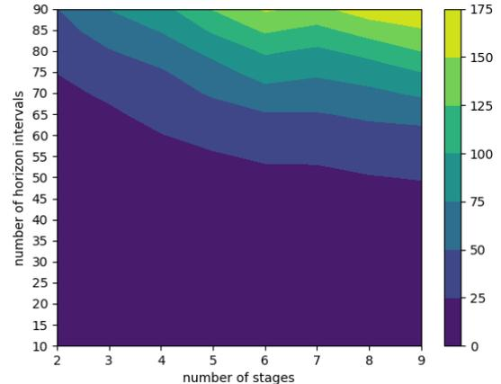
Figure 3.21: Visual representation of the computation times of the PCD algorithm (see Table 3.12).
