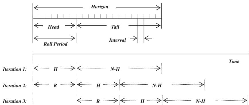
Figure 2.1: A rolling horizon approach for traffic signal control (figure source: [Zheng and Recker, 2013](#)).
