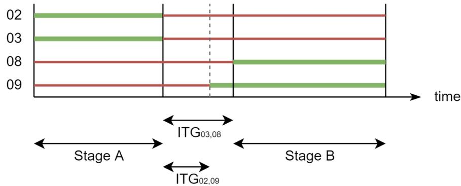
Figure 3.5: The stage-based planning of Figure 3.3 executed via Dutch actuated traffic signal control. The different intergreen times between signal groups allows signal group 09 to become green earlier than signal group 08 and as a result deviations arise between the theoretical planning and the execution of the planning.
