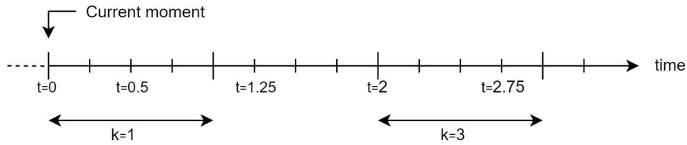
Figure 3.7: The definition of time within the PCD algorithm.  $t$  Represents the real time, which is part of the set of real numbers ( $t \in \mathbb{R}$ ), and  $k$  represents the time index, which is part of the set of natural numbers ( $k \in \mathbb{N}_1$ ).
