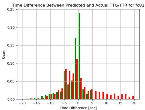
Figure E.37: The TTG and TTR accuracy distribution for signal group 01 in scenario 8 (major-minor, vehicle arrivals).
