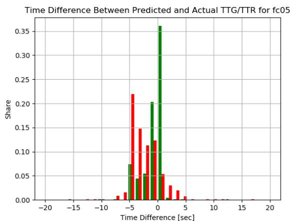
Figure E.40: The TTG and TTR accuracy distribution for signal group 05 in scenario 8 (major-minor, vehicle arrivals).
