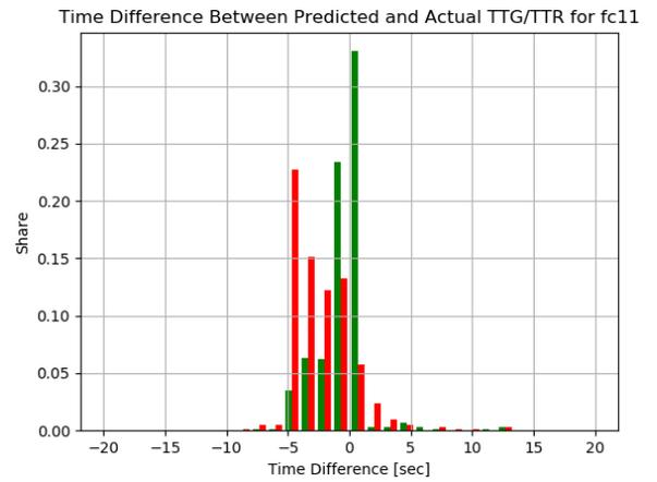
Figure E.34: The TTG and TTR accuracy distribution for signal group 11 in scenario 7 (equal flows, vehicle arrivals).
