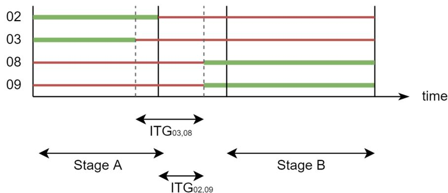
Figure 3.6: The stage-based planning of Figure 3.3 executed via Dutch actuated traffic signal control. The different intergreen times and the early green end of signal group 03 allow signal groups 08 and 09 to realise earlier, and as a result deviations arise between the theoretical planning and the execution of the planning.
