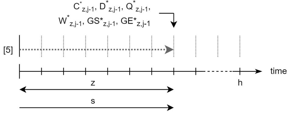
Figure 3.17: In the situation that  $x = 0$ , thus  $s = z$ , no time is allocated to the signal groups of stage  $\varphi = j \bmod N^{\text{stages}}$ , and hence no calculations need to take place. In this situation the delay, queues, green starts time and green ends time equal the solution for limited horizon  $z$  from the previous iteration  $j - 1$ .
