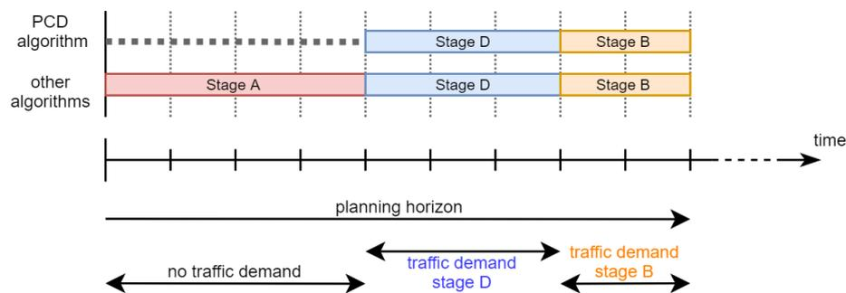
Figure 3.1: The PCD algorithm keeps the planning of control decisions open (gray colour) in case there are no queues and no expected vehicle arrivals. Other algorithms do not include this possibility and they typically dedicate the leftover time to the first stage of the set of stages.
