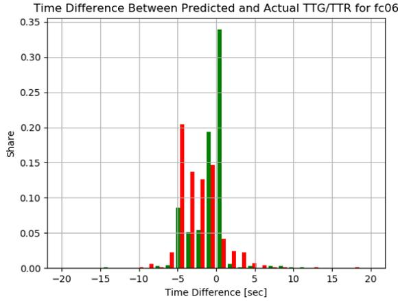
Figure E.41: The TTG and TTR accuracy distribution for signal group 06 in scenario 8 (major-minor, vehicle arrivals).
