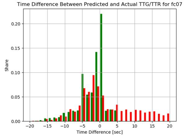
Figure E.42: The TTG and TTR accuracy distribution for signal group 07 in scenario 8 (major-minor, vehicle arrivals).
