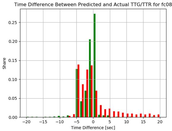
Figure E.43: The TTG and TTR accuracy distribution for signal group 08 in scenario 8 (major-minor, vehicle arrivals).
