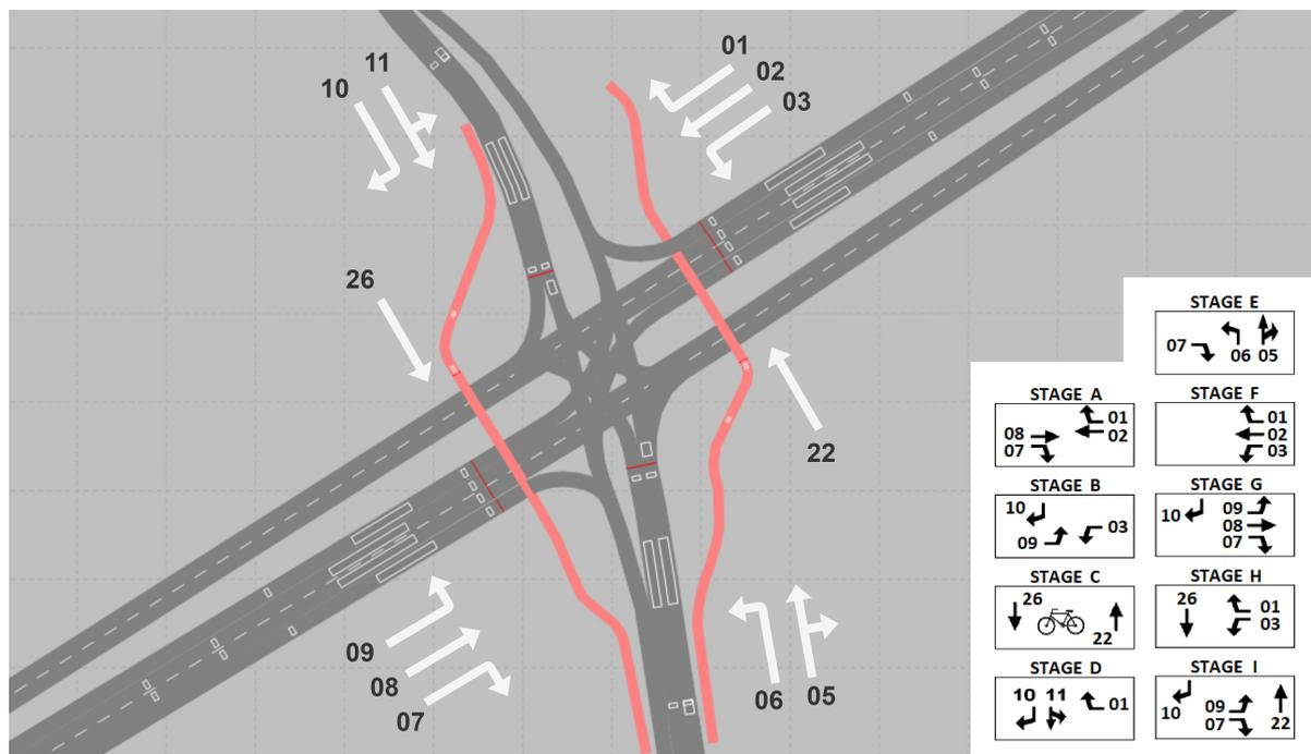
Figure 5.2: The modified Vissim network of the N65 intersection near Helvoirt. The white rectangles represent loop detectors and the red lines represent signal heads. The white arrows and black numbers indicate the present signal groups.
