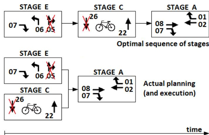
Figure 5.4: An example situation where the sequence of stages presents a distorted view of what is about to happen at the intersection.
