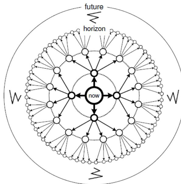
Figure 2.3: An example of a decision tree. All of the circles in the figure represent control decisions (figure source: van Katwijk, 2008).
