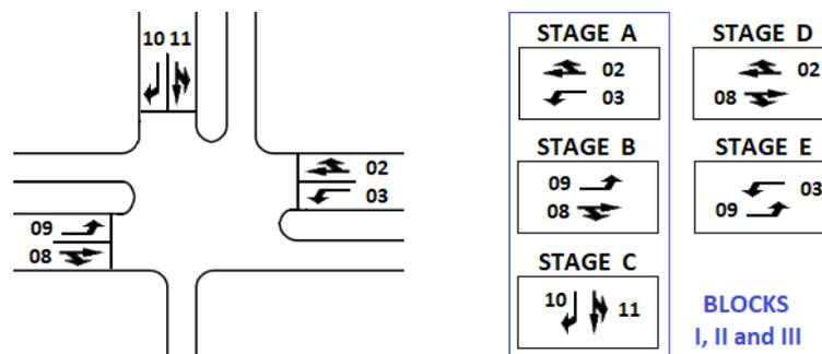
Figure 3.2: An example intersection with corresponding sets of blocks and stages.
