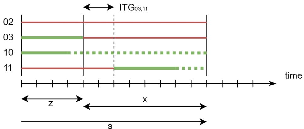
Figure 3.14: The absence of a green request for signal group 02 allows signal group 10 to become green earlier than the start of  $x$ . Green of signal group 10 may even end earlier than the start of  $x$ , as long as the minimum green time constraint for this signal group is met. See the caption of Figure 3.11 for further details.
