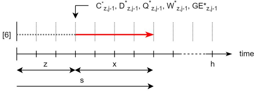
Figure 3.18: The delay is calculated for all time intervals  $k$  that are included in  $x$  (red arrow), taking the queues at the start of  $x$  as a basis. The delay over these intervals is then added to the delay that corresponds to the best performing control policy for limited horizon  $z$  in iteration  $j - 1$  (represented by the broken gray line). This gives the total delay over all time intervals  $k \in \{1, \dots, s\}$ .
