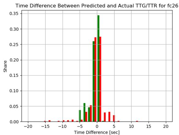
Figure E.36: The TTG and TTR accuracy distribution for signal group 26 in scenario 7 (equal flows, vehicle arrivals).
