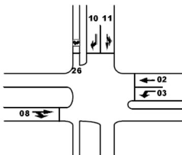
Figure A.2: Standard Dutch coding implemented on a typical intersection (figure source: van Katwijk, 2008).
