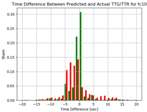
Figure E.45: The TTG and TTR accuracy distribution for signal group 10 in scenario 8 (major-minor, vehicle arrivals).
