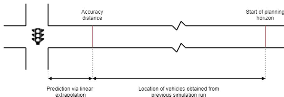
Figure 1.2: Visual representation of the Run and Repeat approach. Between the start of the planning horizon and the accuracy distance the location of vehicles is obtained from the first simulation run. When a vehicle reaches the accuracy distance, prediction of its location takes place via linear extrapolation.
