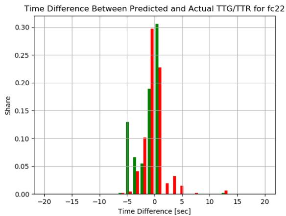
Figure E.47: The TTG and TTR accuracy distribution for signal group 22 in scenario 8 (major-minor, vehicle arrivals).
