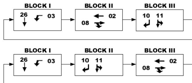
Figure A.3: Two possible block sequences for the intersection of figure A.2. As can be observed, signal groups 08 and 11 have combined directions. This is common practice for intersections with limited streaming areas (figure source: van Katwijk, 2008).
