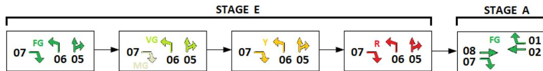
Figure 5.3: An example situation where green of a signal group is ended if that signal group is in two successive stages while there is too low traffic demand. Vehicles that arrive during the amber and red time of signal group 07 experience unnecessary delay, since the signals could technically have stayed green. In the figure time progresses from left to right. The abbreviations of FG, VG, MG, Y and R relate to fixed green, extension green, prolonging green, amber and red respectively.
