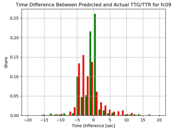
Figure E.44: The TTG and TTR accuracy distribution for signal group 09 in scenario 8 (major-minor, vehicle arrivals).
