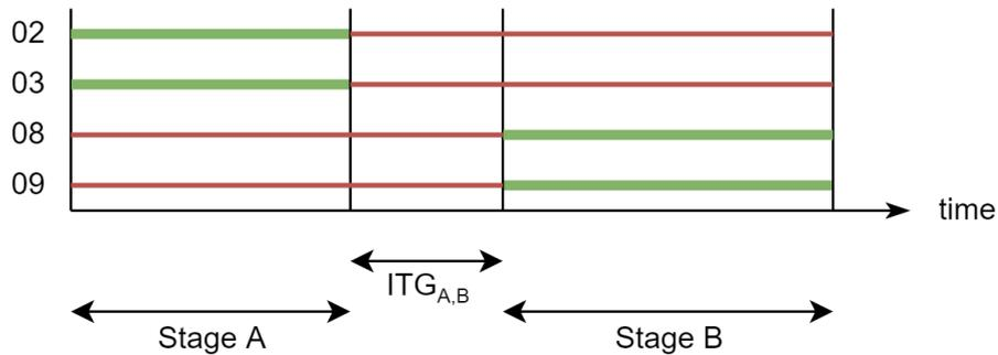
Figure 3.3: An example of a planning of green intervals for signal groups according to a stage-based approach.  $ITG_{A,B}$  denotes the intergreen interval between stages A and B. The green colour denotes green time and the red colour denotes red time. Amber is included in the red time.
