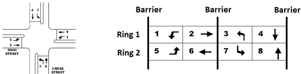
The idea of the ring-barrier structure is that there is always one phase active from either rings and both of the active phases must be located within the same barriers. In total this leaves four phase combinations per barrier group (e.g. 1+5, 1+6, 2+5, 2+6), or eight phase combinations for the entire intersection. The traffic signal controller may only pass a barrier after a user-defined all-red time has elapsed during which all signals at the intersection show red (Rodegerdts et al., 2004).
