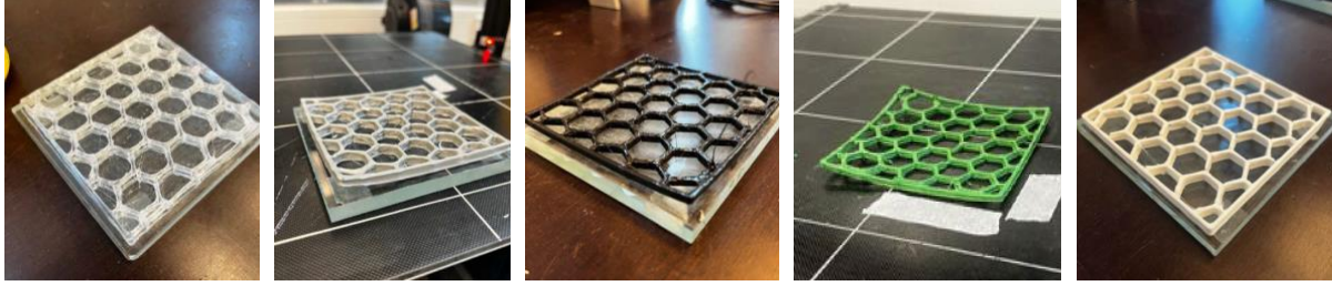
Fig. 3: Samples from left to right: (i) PETG with wood glue exhibiting strong adhesion and no warping; (ii) TPU showing severe warping and poor adhesion; (iii) FlexPolyester with moderate adhesion and corner warping, (iv) PC-ABS that warped of the bed immediately; (v) PLA with high adhesion and no warping
