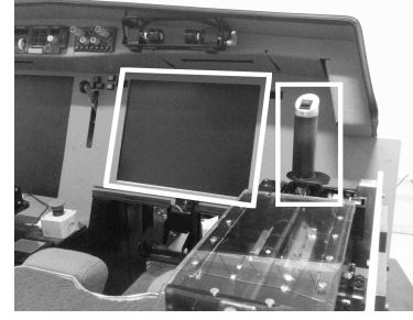
Fig. 2. The apparatus used in the JND experiment. The side-stick manipulator and the LCD screen are marked by white rectangles. The manipulator could be deflected laterally (left/right) like a joystick. The LCD screen only displays the visual presentation of the tracking task.
