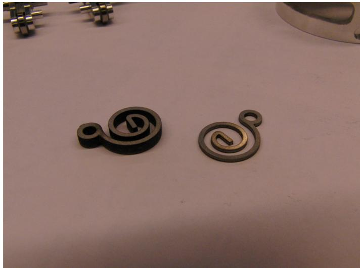
Figure 5.5: Torsion spring in reality. These springs were laser cut from 1 mm RVS301 stainless springsteel and from 3 mm RVS301 sltainless springsteel. The slotted axle connection and the pin follower connection can be seen in this photo.
