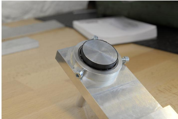
Figure D.1: The braking disk produced from Alu7075 with braking rubber glued on the outer surface.
