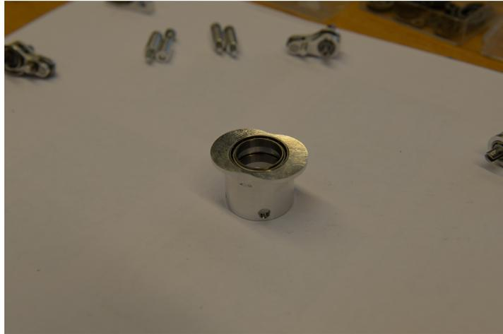
Figure D.6: Cam disk produced in Alu7075 to the matlab model. Two thin section ball bearings are incorporated to deal with the forces and moments exerted on the cam surface.
