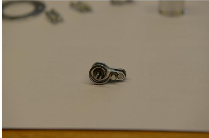
Figure D.9: Follower link with spring attached. The follower is machined from Alu7075 and features three roller bearings. One to roll over the cam surface, and two on the main axle to compensate for the load introduced by the torsion spring.
