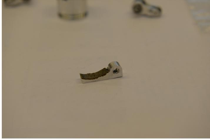
Figure D.2: The braking lever produced from Alu7075 with braking material glued on the inner surface.
