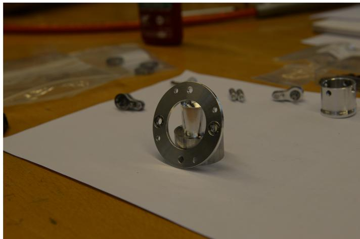
Figure D.8: Secondary body machined from Alu7075.
