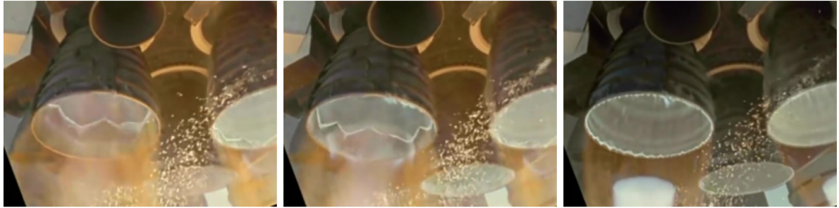
Figure 1.2: Transient start-up of the SSME. Figures obtained from NASA (Pasquariello, 2018).
