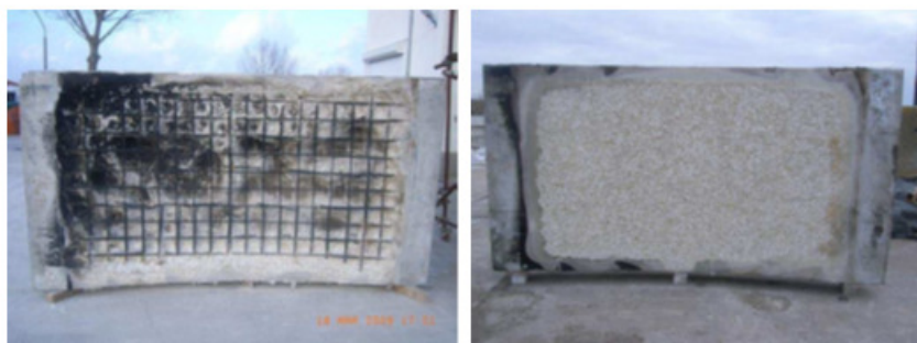
Figure 8: Spalling without (left) and with (right) inclusion of PP fibers in the mixture [15]
