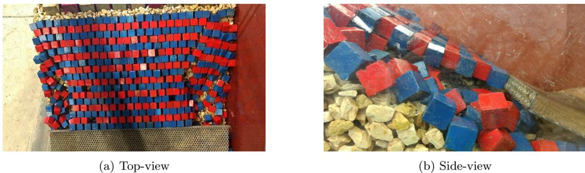
Figure 4.9: Photo's of the hollow space under the armour layer of the configuration with a fixed toe
