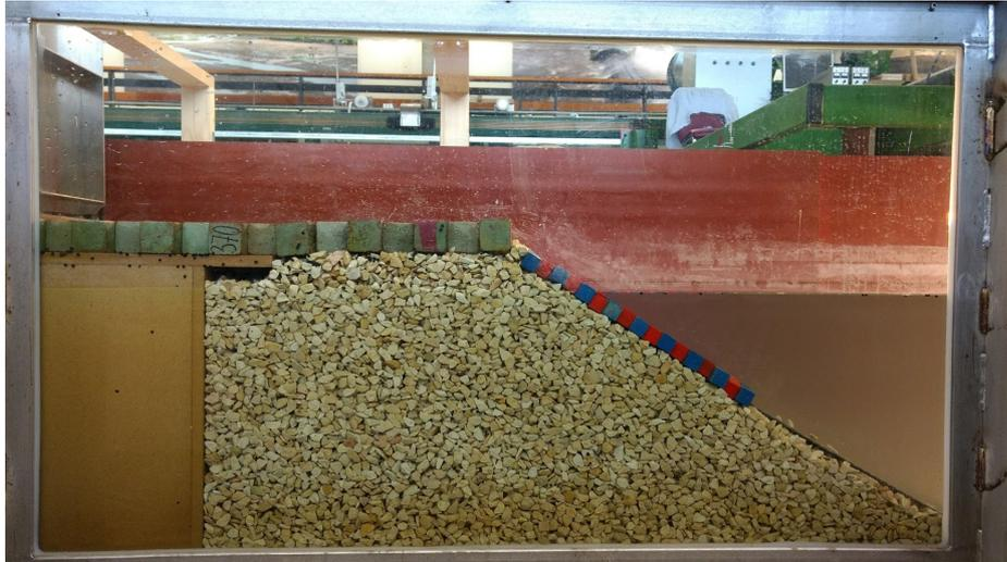
Figure 4.8: Test set-up built with a fixed toe
