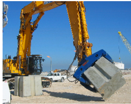
Figure 2.9: Hydraulic clamping system
