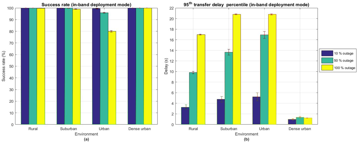
**Figure 6-3. Comparison, for different environments in an in-band deployment mode, of (a) the success rate and (b) the 95<sup>th</sup> transfer delay percentile. The error bars indicate the 95 % confidence intervals of the mean value obtained across 100 simulation snapshots.**
