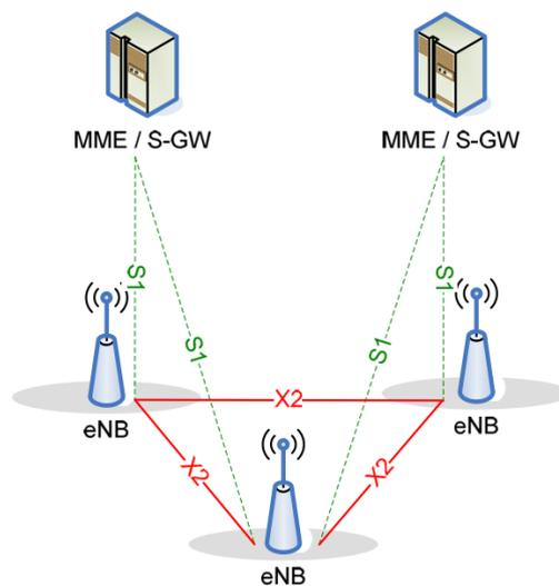
Figure 3-1. NB-IoT access network design [40].
