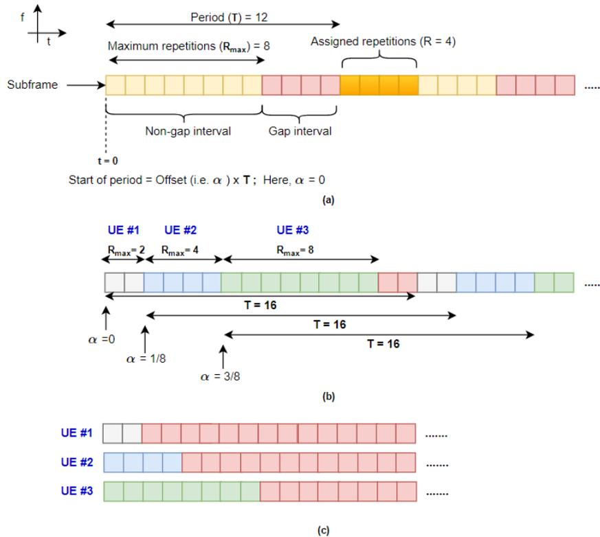
Figure 3-11. Illustration of (a) an example NPDCCH configuration for a UE, (b) the use of the offset ( $\alpha$ ) to create non-overlapping NPDCCH configurations and (c) a corresponding overlapping NPDCCH configuration.
