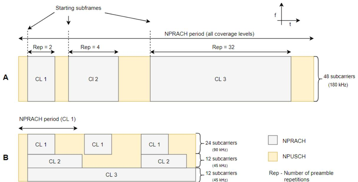
Figure 3-16. Example NPRACH resource configurations (A and B) for three Coverage Levels (CLs).
