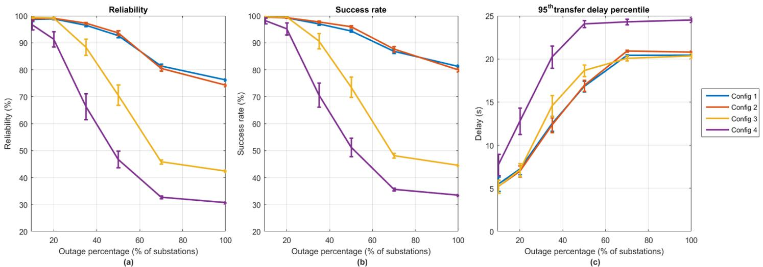
Figure 6-5. Comparison of (a) the reliability, (b) the success rate and (c) the 95<sup>th</sup> transfer delay percentile among the considered NPRACH resource configurations.
