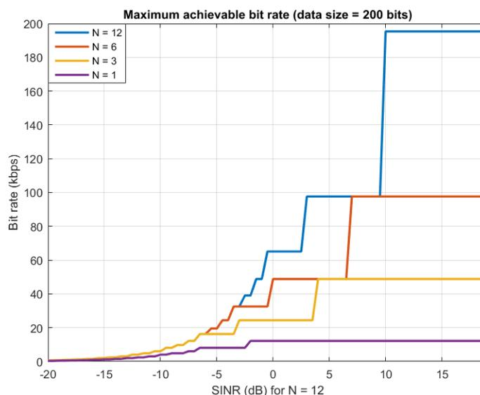
Figure 5-3. Comparison of the maximum achievable bit rate using a data size of 200 bits for different number (N) of assigned subcarriers.
