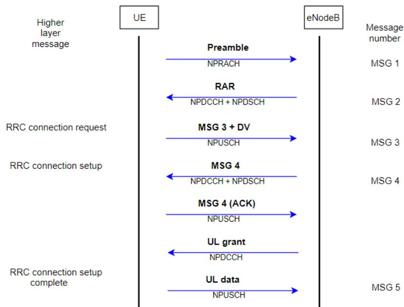
Figure 3-13. Random access procedure call flow in NB-IoT. The corresponding higher layer message is indicated on the left and the message number indicated on the right.
