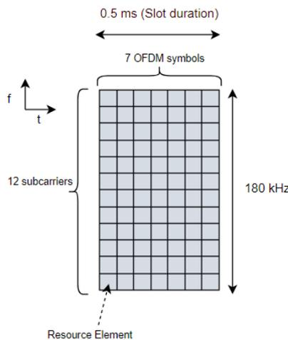
Figure 3-3. NB-IoT downlink resource grid.
