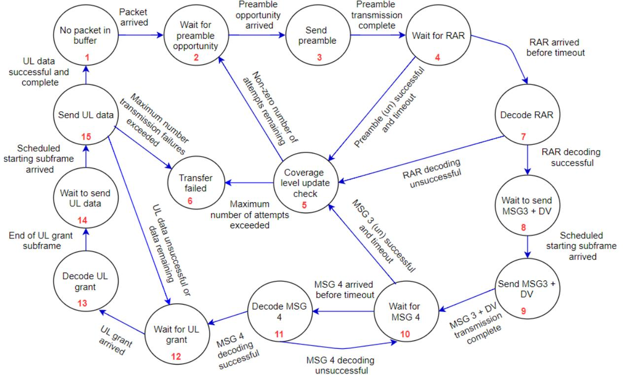
Figure 4-3. Event-driven state transitions for a UE attempting to send uplink data.
