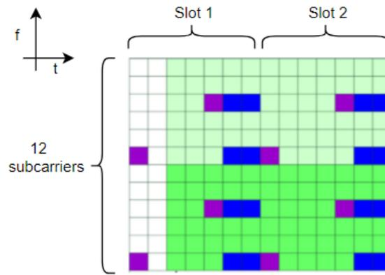
Figure 3-10. An NPDCCH subframe (in an in-band deployment) with two NCCes (in light and dark green). The violet and blue resource elements correspond to the LTE and the NB-IoT reference signals respectively. The white-coloured resource elements are reserved for the LTE control channel known as the PDCCH.
