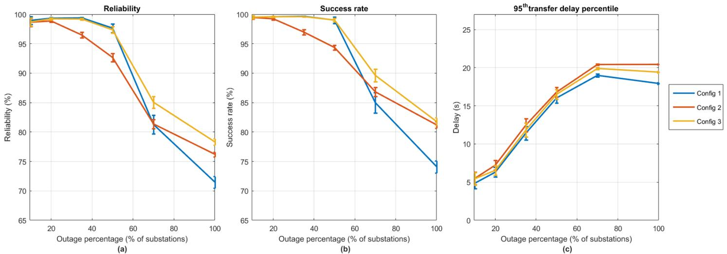
Figure 6-9. Comparison of (a) the reliability, (b) the success rate and (c) the 95<sup>th</sup> transfer delay percentile among the candidate quasi-optimal configurations.
