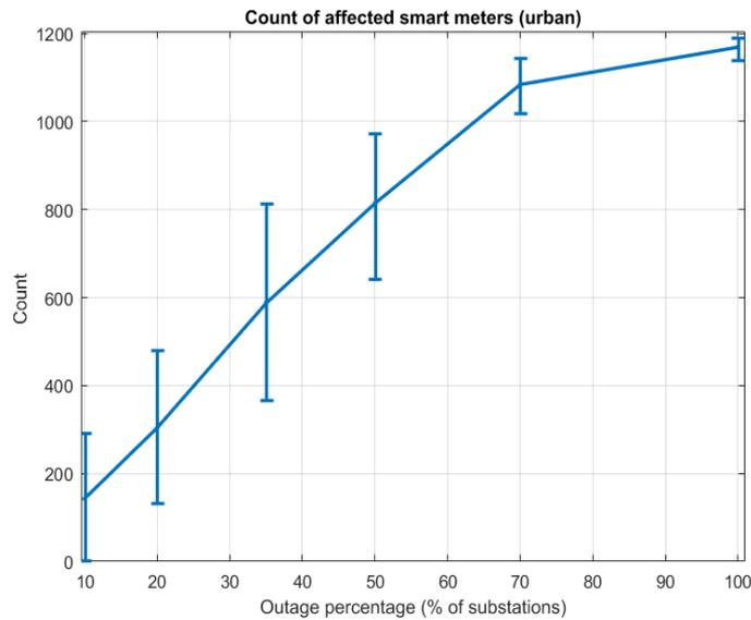
Figure 6-4. Count of affected smart meters, in the urban environment, for the outage percentages considered in the sensitivity analysis. The data points and error bars indicate the mean and standard deviation, respectively, of the obtained values across 100 simulation snapshots.
