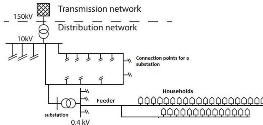
**Figure 4-5. General energy distribution network topology in The Netherlands [56]. The different substations are connected in a ring. Feeders connect different households in a radial topology.**
