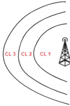
Figure 3-15. Simplified spatial representation of different coverage levels around the base station (CL stands for coverage level).
