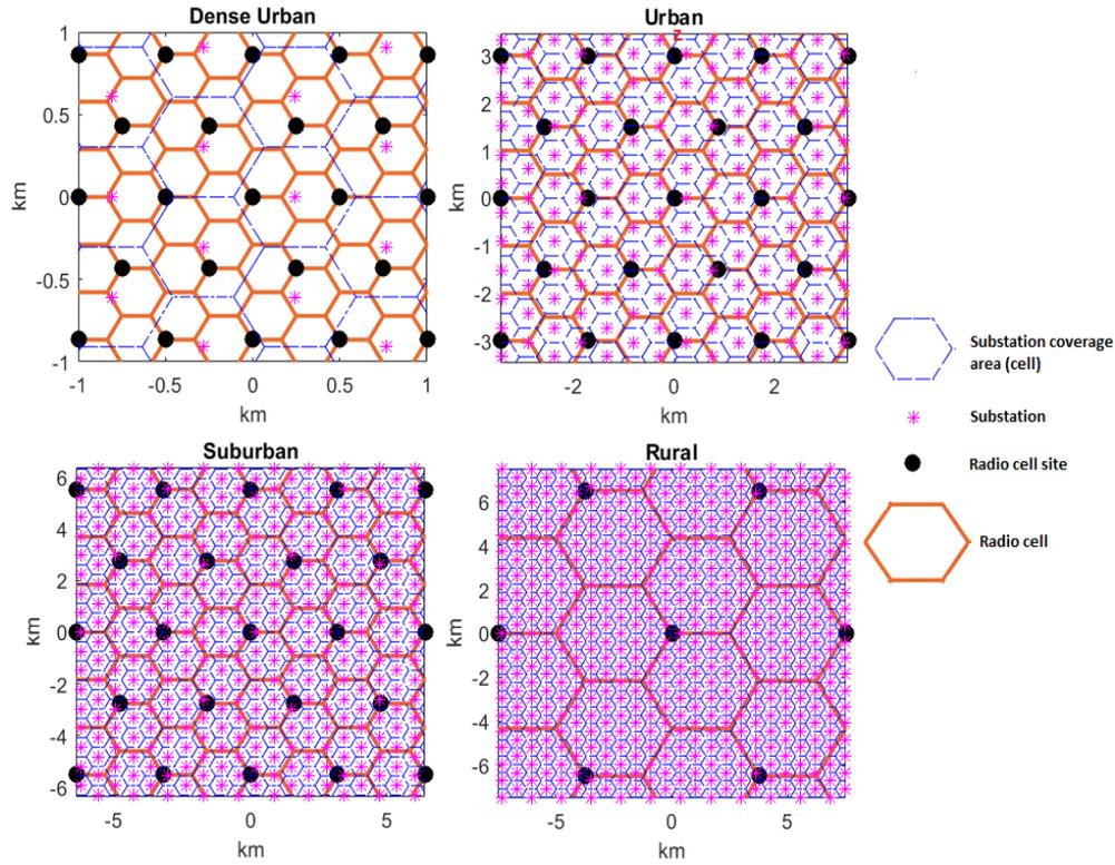
Figure 4-6. Radio network and energy distribution network layout for different environments.
