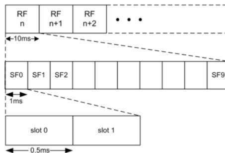
Figure 3-4. Downlink radio frame structure in NB-IoT (RF stands for radio frame, SF for subframe) [46].
