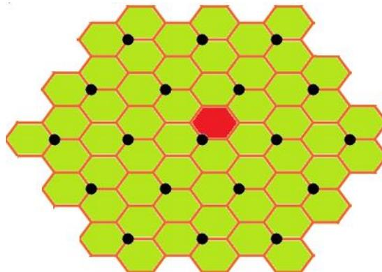
**Figure 4-4.** Hexagonal grid of radio cells. Cell sites are represented by the black markers. The simulation is executed for only UEs in the radio coverage of the red cell. The green cells represent the interfering cells.
