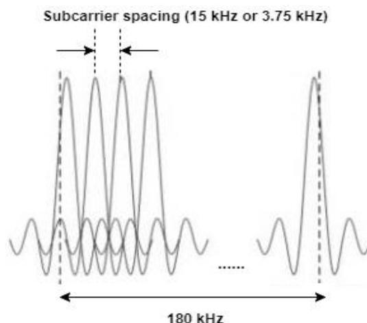
Figure 1-3. NB-IoT bandwidth of 180 kHz consisting of orthogonal subcarriers.
