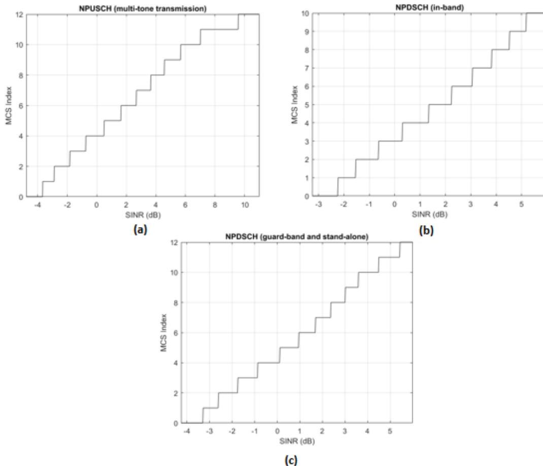
Figure E-1. SINR-MCS step functions for (a) the NPUSCH (multi-tone transmission), (b) the NPDSCH (in-band deployment mode) and (c) the NPDSCH (guard-band and stand-alone deployment modes).
