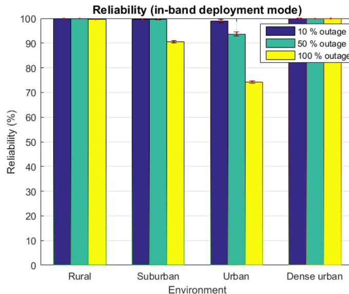
Figure 6-2. Comparison of the reliability performance for each environment under an in-band deployment mode. The error bars indicate the 95 % confidence intervals of the mean value obtained across 100 simulation snapshots.
