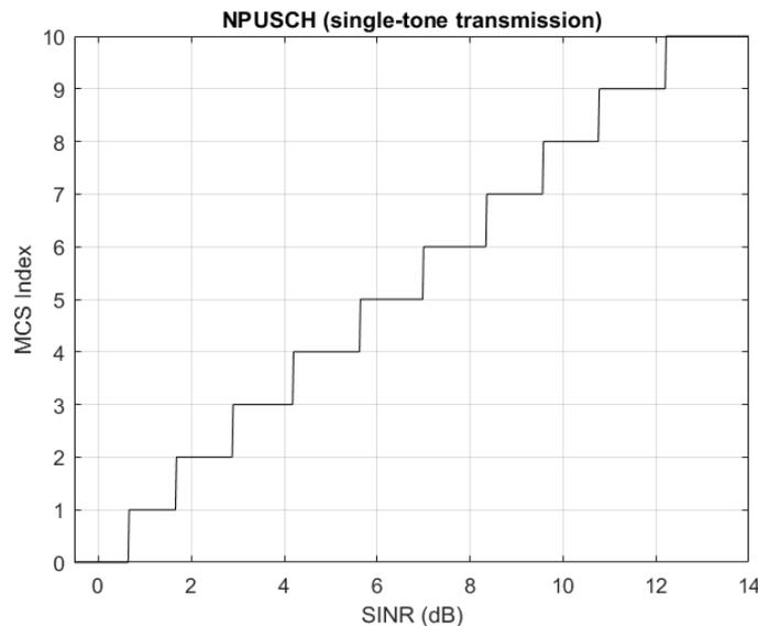
**Figure 4-8. SINR-MCS step function (for NPUSCH single-tone transmission).**
