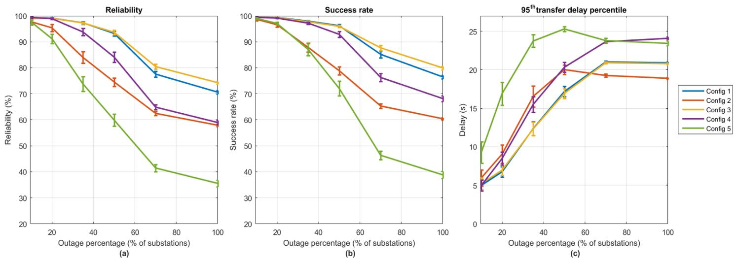
Figure 6-7. Comparison of (a) the reliability, (b) the success rate and (c) the 95<sup>th</sup> transfer delay percentile among the considered schedulers.
