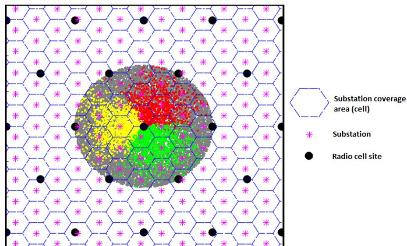
**Figure 4-7. Radio and energy distribution network coverage map for a region around the central site, shown for an urban environment.**
