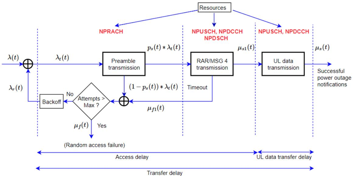
Figure 5-1. Illustration of a simplified traffic flow within the random access process and the uplink data transmission that follows, from a system perspective.
