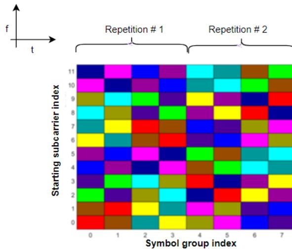
**Figure 3-14. Example NPRACH preamble transmission. There are twelve starting subcarriers i.e. preambles, and each colour represents a different frequency hopping sequence.**
