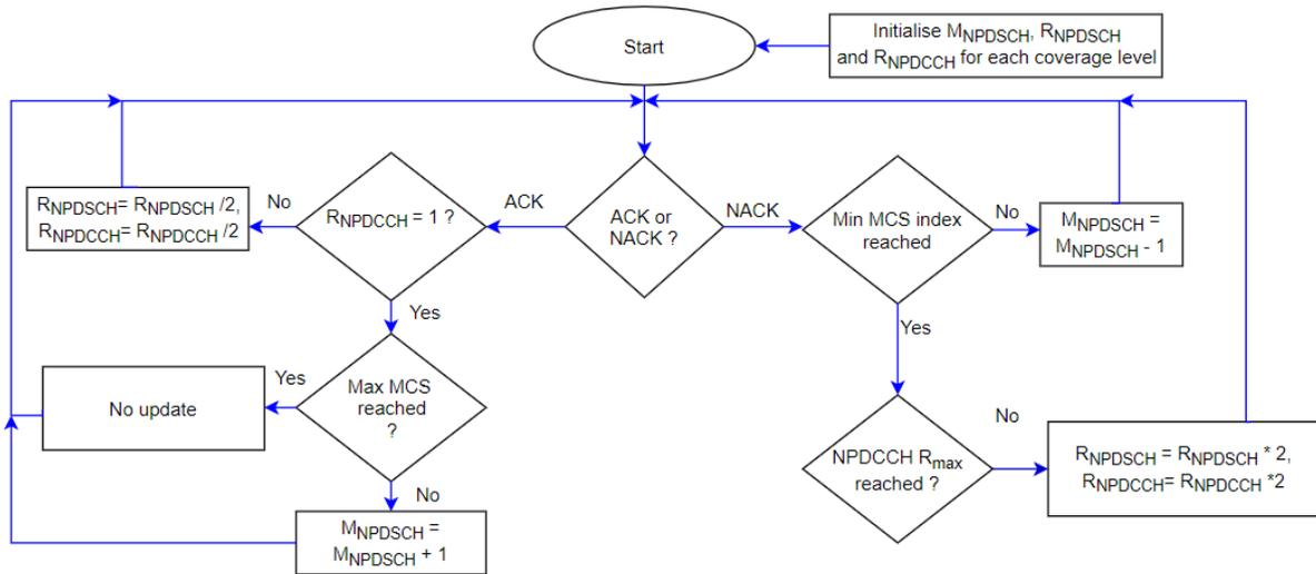
Figure 4-9. Link adaptation flow diagram.
