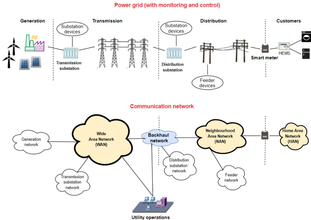
Figure 1-5. A conceptual representation of a smart grid in terms of the power grid and the related communication network connecting various monitoring and control devices [8].
