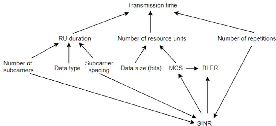
Figure 3-7. Relationship between parameters which determine the uplink transmission time and BLER for a UE.
