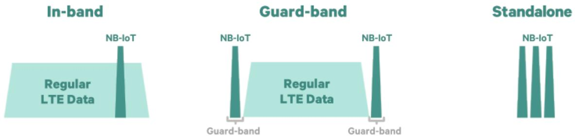
Figure 1-4. The different carrier deployment options in NB-IoT [6].
