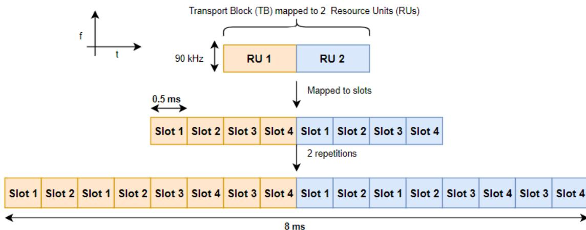
Figure 3-8. Example transmission of an uplink transport block using six subcarriers (15 kHz subcarrier spacing), two resource units and two repetitions.
