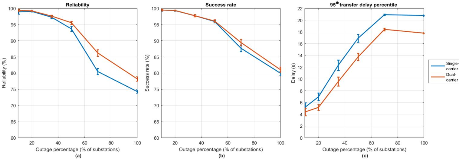
Figure 6-10. Comparison of (a) the reliability, (b) the success rate and (c) the 95<sup>th</sup> transfer delay percentile among a single-carrier and dual-carrier operation.
