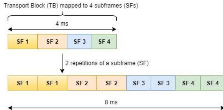
Figure 3-5. Example of downlink transmission of a transport block mapped to four subframes with two repetitions.
