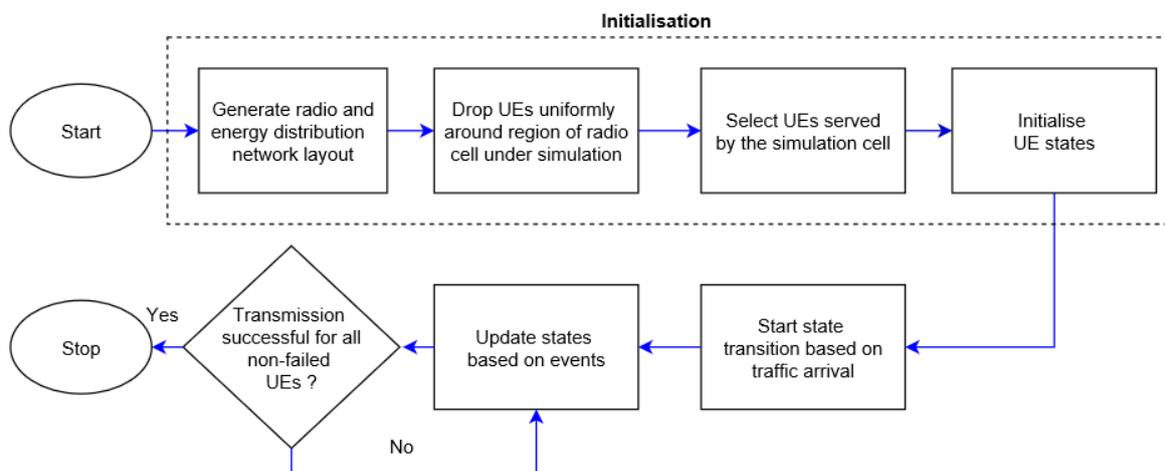
Figure 4-2. High-level simulation flow per simulation snapshot.
