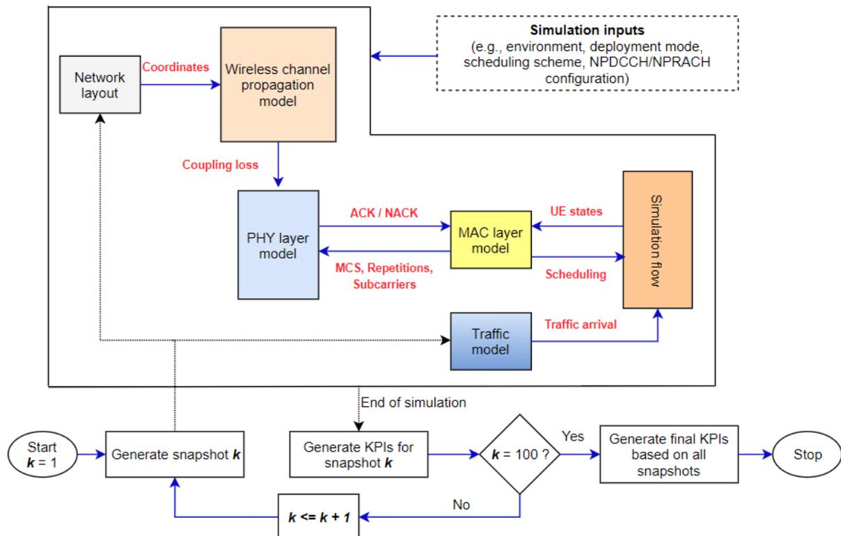
Figure 4-1. Overview of simulation process and the interaction between the six components (encircled) of the NB-IoT simulation model.
