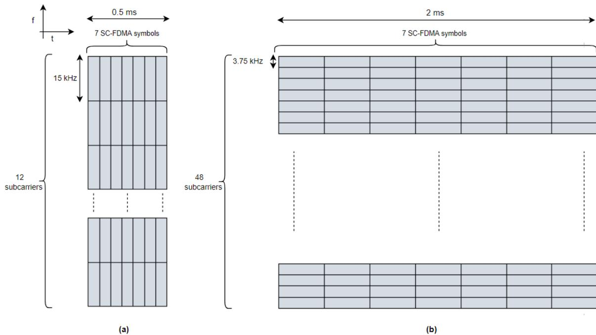
Figure 3-6. NB-IoT uplink resource grid for (a) 15 kHz and (b) 3.75 kHz subcarrier spacing.
