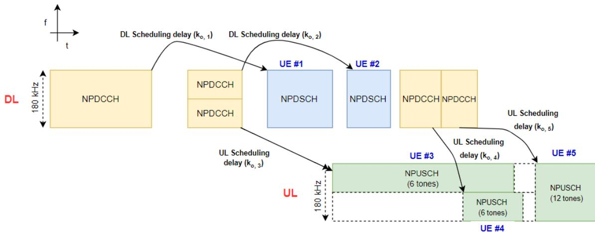
Figure 3-12. Illustration of a generic scenario of DL (top) and UL (bottom) scheduling of UEs in NB-IoT.
