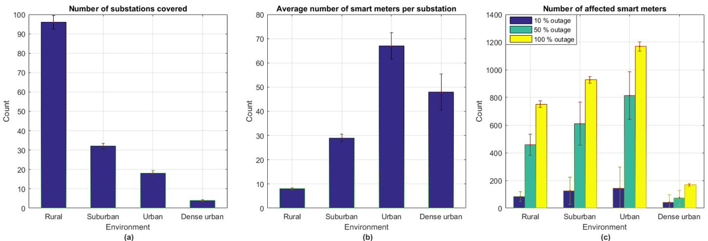
Figure 6-1. Plots showing, for each environment, (a) the number of substations covered in the radio cell, (b) the average number of smart meters per substation and (c) the number of smart meters affected by different outage percentages. The bar values and error bars indicate the mean and standard deviation, respectively, of the obtained values across 100 simulation snapshots.
