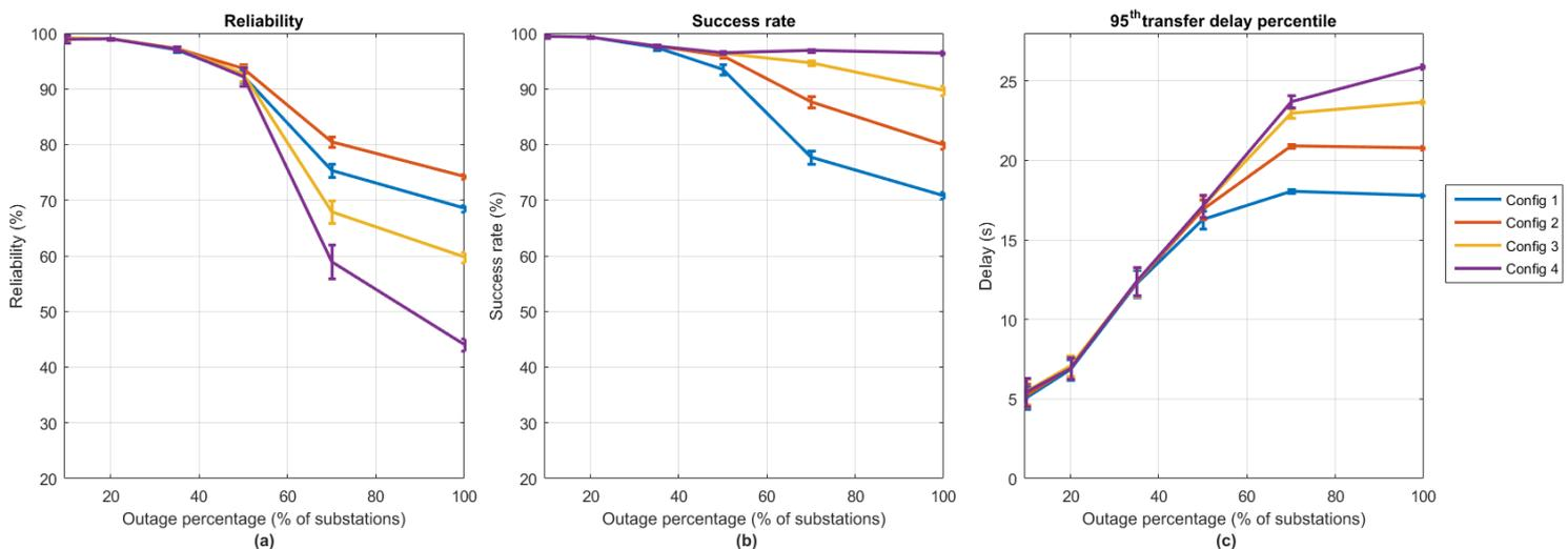
Figure 6-6. Comparison of (a) the reliability, (b) the success rate and (c) the 95<sup>th</sup> transfer delay percentile among the considered configurations of the maximum number of RA attempts.
