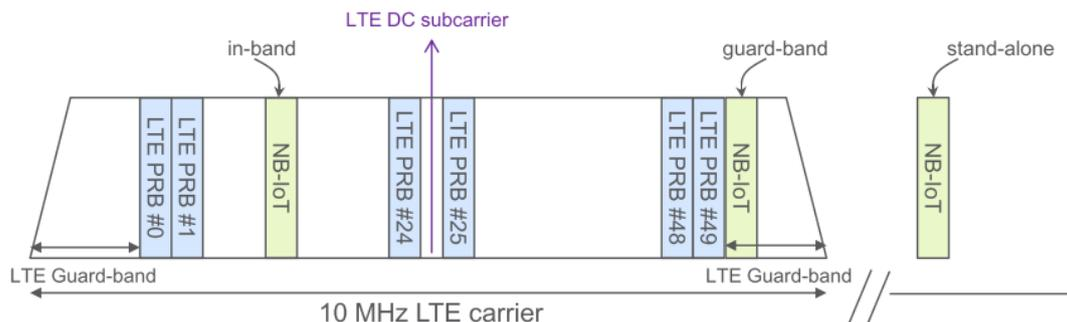
Figure 3-2. Different carrier deployment options for NB-IoT [42].
