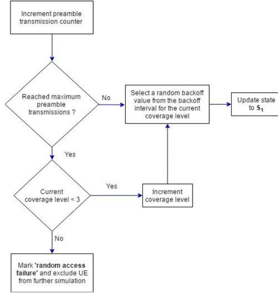
Figure A-4. Coverage level update procedure (for states 3, 4 and 7).
