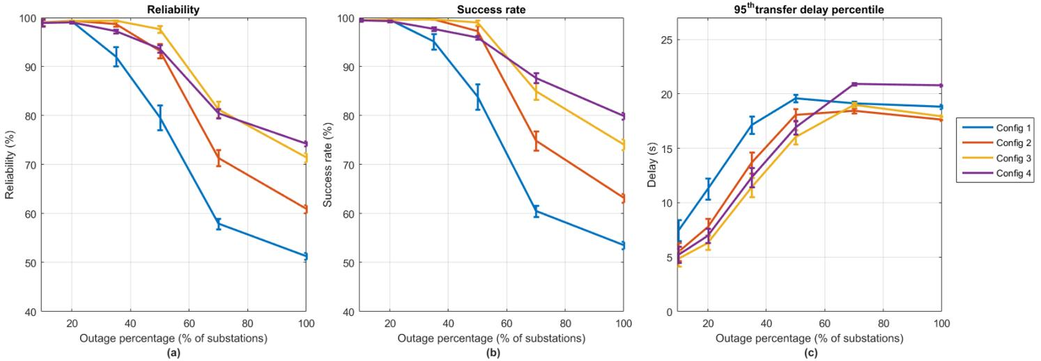
Figure 6-8. Comparison of (a) the reliability, (b) the success rate and (c) the 95<sup>th</sup> transfer delay percentile among the considered NPDCCH resource configurations.
