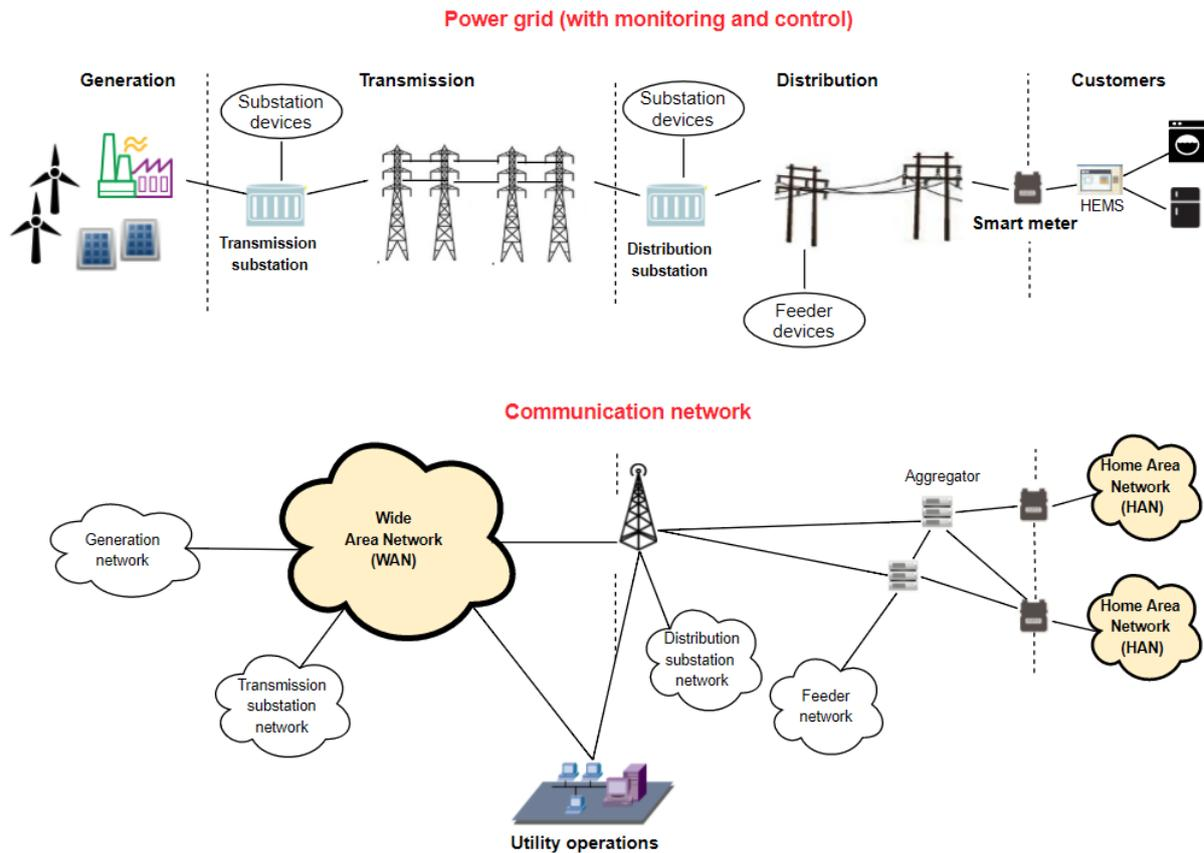
**Figure 2-1. Representation of the hierarchical smart grid communication network in relation with the different power grid segments and various monitoring and control devices.**
