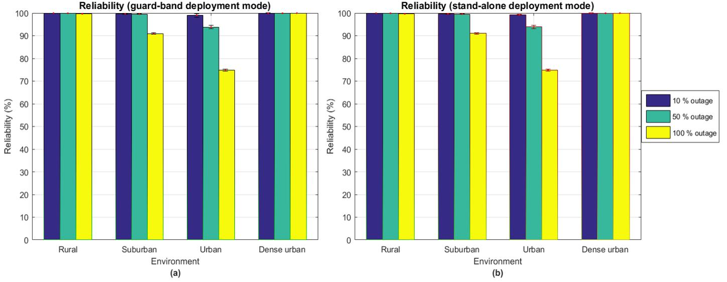
Figure F-1. Comparison of the reliability performance with the baseline configuration for different environments under (a) the guard-band and (b) the stand-alone deployment modes of NB-IoT.
