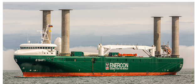
(b) E-ship 1 (2010) equipped with four rotor sails and top end plates ( H=27.0 [m], D=4.0 [m]). Reproduced from Wikimedia Commons Contributors (2025).
