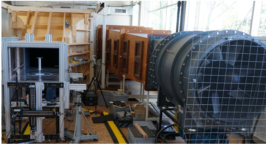
Figure 3.8: Overview of wind tunnel with test section and traverse system, barriers and operators location.
