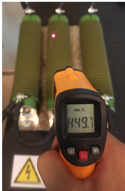
Figure 3.22: Resistors test showing a temperature of 449 °C.
