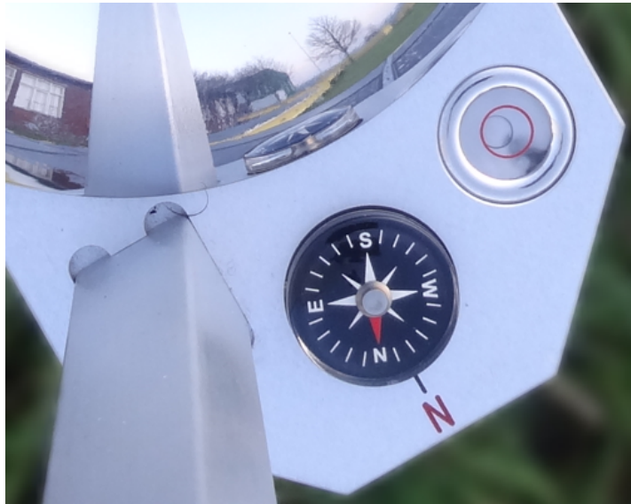
Figure E.18: Horicatcher orientation and inclinations taken into account during horizon measurement on-land.
