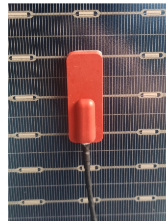
(b) PT100 sensor installed on PV modules on-land and off-shore.
