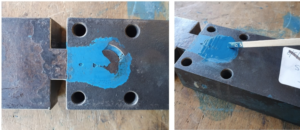
Figure 3.16: a. Hole clearance not completely filled by resin b. Further addition of resin into the hole clearance
