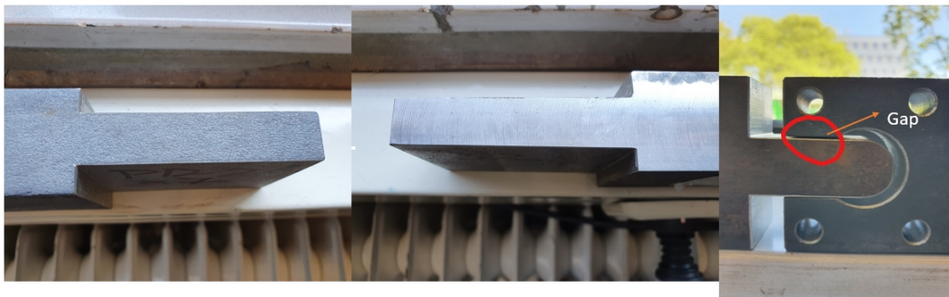
Figure 3.13: Geometrical imperfections due to manufacturing tolerances
