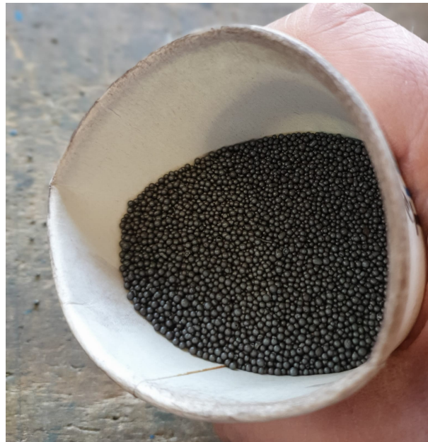
Figure 3.7: Spherical steel shots (S330) with diameter of 0.84 mm
