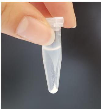
**Figure 5.1:** Eppendorf tube for the detection of hydrogen peroxide immediately after being centrifuged for 30 minutes at 10,000 rpm. The solution was still relatively cloudy, meaning that a large fraction of the nanoparticles was not precipitated.
