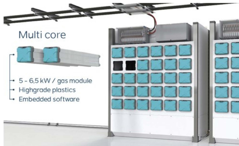
Figure 1.7: XINTC Hydrogen Gas Modules. A single gas module is approximately 25 cm wide and tall, and 60 cm long, with a nominal power of 5-6.5kW. Two modules operate in pairs. Scalable solutions are achieved by adding sections of gas modules together. This modular system design is one of the first of its kind and makes XINTC a pioneer in the mid-market electrolyzer industry [47]. Permission was obtained by XINTC for the use of this image.
