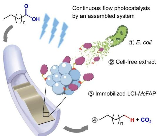
This is an assembled photoenzyme-loaded membrane mesoscale reactor based on the behavior of biomole-
