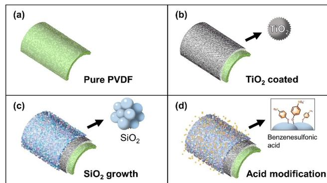
**Scheme 2.** Design of functionalized membranes. (a) PVDF membrane as support (pore size 0.45  $\mu\text{m}$ ); (b)  $\text{TiO}_2$  coating provided active hydroxyl groups and nucleation sites, PVDF-Ti; (c) in situ growth of  $\text{SiO}_2$  nanoscale particles to increase the effective surface area, PVDF-Ti-Si; (d) covalent coating with 4-chlorobenzene sulfonic acid to attain overall negatively charged surfaces, PVDF-Ti-Si- $\text{SO}_3\text{H}$ .
