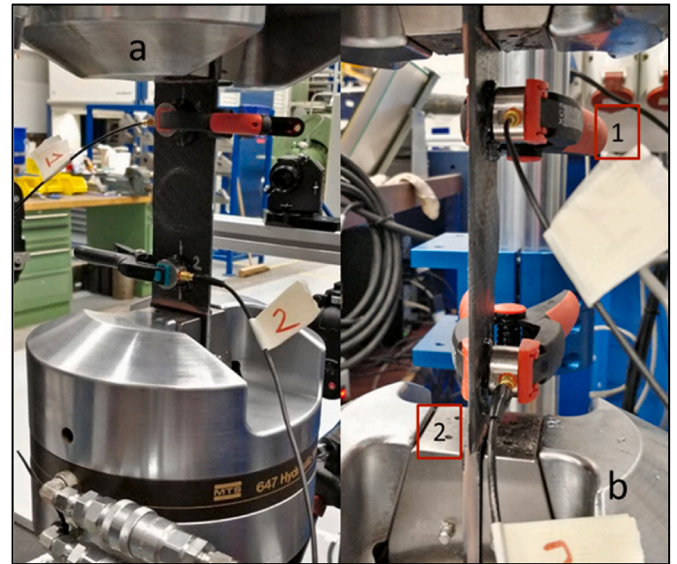
Fig. 10. Acoustic emission sensors positioned during the Tensile tests a) back view b) side view.
