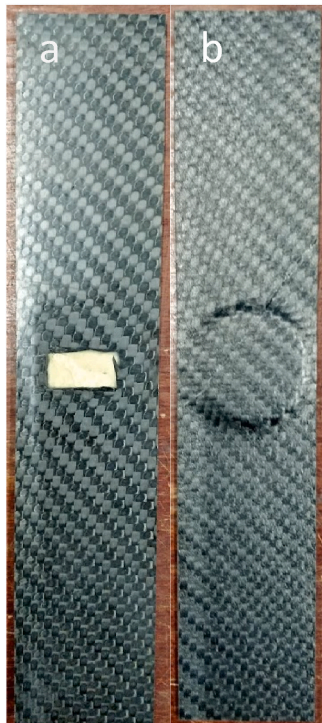
Fig. 5. Image of tensile composite specimens a) front and, b) back.
