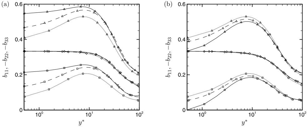
FIG. 9. Profiles of normal Reynolds stress anisotropies as a function of  $y^*$  for (a) case GL and (b) case LL, compared to CP395 and Iwamoto, Suzuki, and Kasagi.<sup>32</sup> In (a) and (b): ( $\Delta$ )  $b_{11}$ , ( $\diamond$ )  $b_{22}$ , ( $\square$ )  $b_{33}$ . Lines are the same as in Figure 7.
