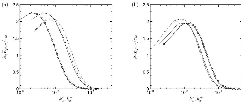
FIG. 12. Comparison of pre-multiplied 1D stream-wise spectra of  $\overline{\rho u''u''}/\tau_w$  at  $y^* \approx 15$  for (a) case GL and (b) case LL. Lines with symbols are plotted as function of  $k_x^+$ , while lines without symbols are plotted as function of  $k_x^*$ . Lines are the same as in Figure 7.
