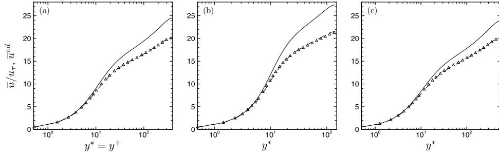
FIG. 3. Averaged velocity profiles for cases (a) CP395 and  $CRE_{\tau}^*$ , (b)  $SRE_{\tau GL}^*$  and GL, (c)  $SRE_{\tau Cv}^*$  and Cv. Symbols are constant density cases: CP395,  $SRE_{\tau GL}^*$ , and  $SRE_{\tau Cv}^*$ , lines are variable density cases:  $CRE_{\tau}^*$ , GL, and Cv. (—) mean stream-wise velocity  $\bar{u}/u_{\tau}$  and (- - -) van Driest transformed stream-wise velocity profile  $\bar{u}^{vd}$ .
