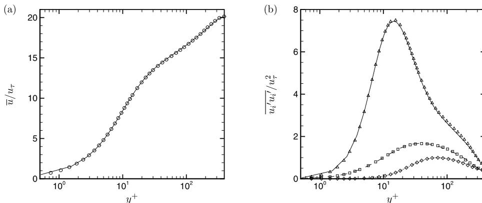
FIG. 18. (a) Mean velocity profile and (b) normal Reynolds stresses. Lines, case CP395; symbols, data from Moser, Kim, and Mansour.<sup>2</sup> In (b), (—,  $\Delta$ )  $\overline{u'u'}$ ; ( $\cdots$ ,  $\diamond$ )  $\overline{v'v'}$ ; (- - -,  $\square$ )  $\overline{w'w'}$ .
