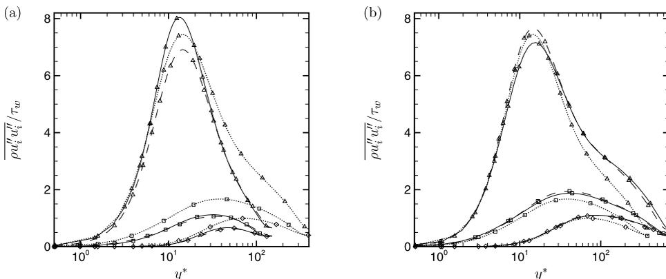
FIG. 8. Profiles of normal Reynolds stresses as a function of  $y^*$  for (a) case GL and (b) case LL, compared to CP395 and Iwamoto, Suzuki, and Kasagi.<sup>32</sup> Lines and symbols are the same as in Figure 7.
