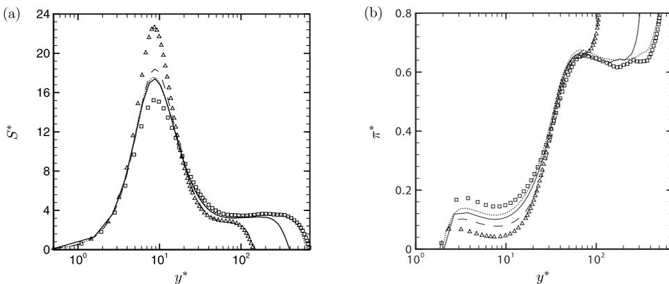
FIG. 14. (a) The turbulence-to-mean time scale ratio  $S^*$  and (b) pressure strain to production ratio  $\pi^*$  of  $\overline{\rho u'' u''} / \tau_w$  for case GL and case LL, compared with CP395 and Iwamoto, Suzuki, and Kasagi.<sup>32</sup> ( $\Delta$ ) case GL, ( $\square$ ) case LL, (—) case CP395, (---)  $h^+ = 150$  from Iwamoto, Suzuki, and Kasagi<sup>32</sup> and (.....)  $h^+ = 650$  from Iwamoto, Suzuki, and Kasagi.<sup>32</sup>
