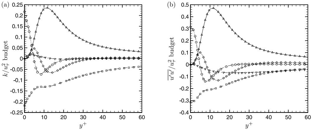
FIG. 19. (a) Turbulent kinetic energy  $k = \overline{u_k' u_k'}/(2u_\tau^2)$  budget and (b) stream-wise Reynolds stress  $\overline{u'u'}/u_\tau^2$  budget. Lines, case CP395; symbols, data from Moser, Kim, and Mansour.<sup>2</sup> (—,  $\Delta$ ) Production; (---,  $\square$ ) dissipation; ( $\cdots$ ,  $\diamond$ ) turbulent diffusion; (— · —,  $\circ$ ) viscous diffusion; (— · —,  $\nabla$ ) turbulent pressure diffusion in (a) and pressure strain in (b).
