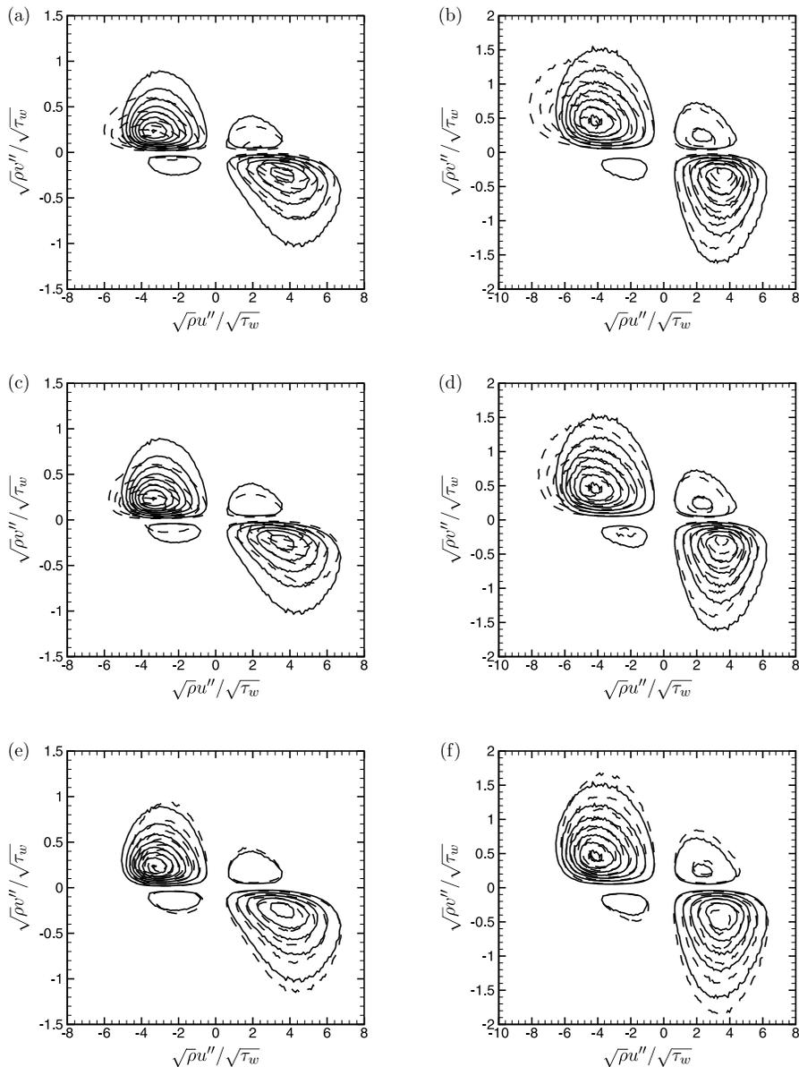
FIG. 17. Joint pdf of  $\sqrt{\rho u''}/\sqrt{\tau_w}$  and  $\sqrt{\rho v''}/\sqrt{\tau_w}$  with contours of probability weighted Reynolds shear stress  $\rho u''v''/\tau_w P(\sqrt{\rho u''}/\sqrt{\tau_w}, \sqrt{\rho v''}/\sqrt{\tau_w})$ , for (a) and (b) case GL, (c) and (d) case  $SRe_{\tau_{GL}}^*$ , and (e) and (f) case LL, compared with CP395. Left column  $y^* \approx 8.5$ ; right column  $y^* \approx 15$ . (—) Case CP395, (---) case GL, (· · ·) case  $SRe_{\tau_{GL}}^*$ , LL.
