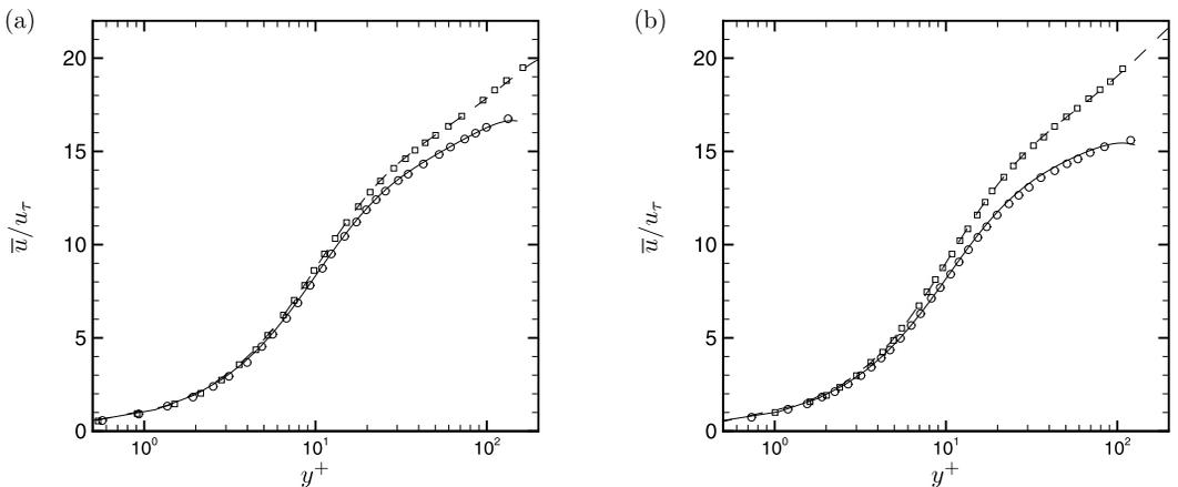
FIG. 21. Mean velocity profile for case with (a)  $T_2/T_1 = 2$  and (b)  $T_2/T_1 = 4$ . Lines, present code; symbols, data obtained from Nicoud.<sup>24</sup> (—,  $\circ$ ) Hot side; (---,  $\square$ ) cold side.
