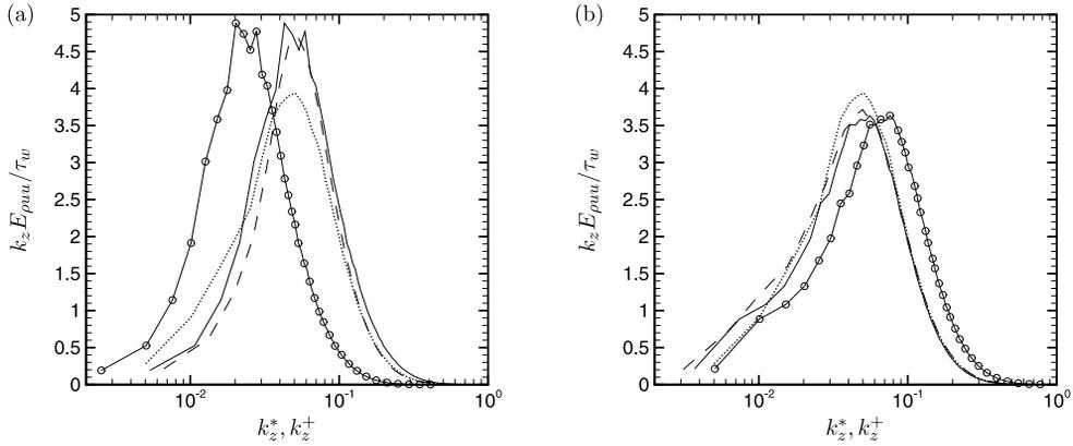
FIG. 13. Comparison of pre-multiplied 1D span-wise spectra of  $\overline{\rho u'' u''} / \tau_w$  at  $y^* \approx 15$  for (a) case GL and (b) case LL. Lines with symbols are plotted as function of  $k_z^+$ , while lines without symbols are plotted as function of  $k_z^*$ . Lines are the same as in Figure 7.
