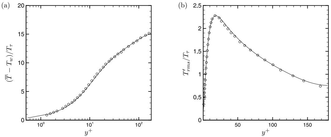
FIG. 20. (a) Mean temperature profile  $(\overline{T} - T_w)/T_\tau$  and (b) root mean square of temperature fluctuations  $T'_{rms}/T_\tau$ ,  $T_\tau$  is friction temperature defined as  $T_\tau = q_w/(\rho c_p u_\tau)$ . Lines, present code; symbols, data obtained from Kim and Moin.<sup>16</sup>
