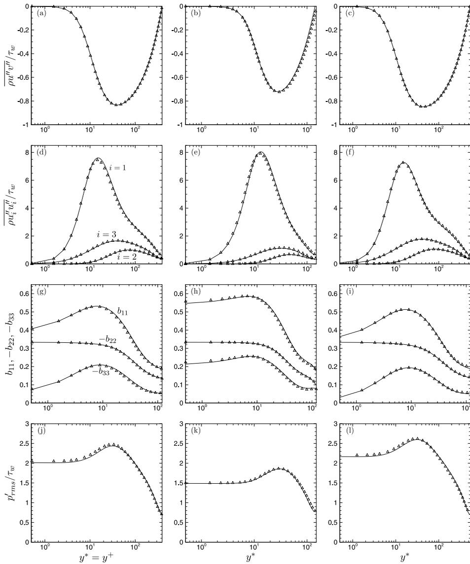
FIG. 4. Comparison of ((a)-(c)) Reynolds shear stress, ((d)-(f)) normal Reynolds stresses, ((g)-(i)) normal Reynolds stress anisotropies, and ((j)-(l)) root mean square of pressure fluctuations for cases (left column) CP395 and  $CRE_{\tau}^*$ , (middle column)  $SRE_{\tau GL}^*$  and GL, (right column)  $SRE_{\tau Cv}^*$  and Cv. Symbols are constant density cases: CP395,  $SRE_{\tau GL}^*$ , and  $SRE_{\tau Cv}^*$ , lines are variable density cases:  $CRE_{\tau}^*$ , GL, and Cv.
