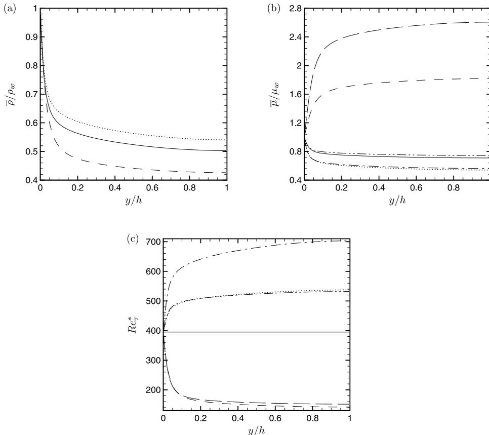
FIG. 1. (a) Density  $\bar{\rho}/\rho_w$ , (b) viscosity  $\bar{\mu}/\mu_w$ , and (c) local Reynolds number  $\text{Re}_\tau^* = h/\delta_v^*$ . (—)  $\text{CRe}_\tau^*$ , (---) GL, (— · —) LL, (·····)  $\text{Cv}$ , (— · — ·)  $\text{SRe}_{\tau\text{Cv}}^*$ , (— · — ·)  $\text{SRe}_{\tau\text{GL}}^*$ .
