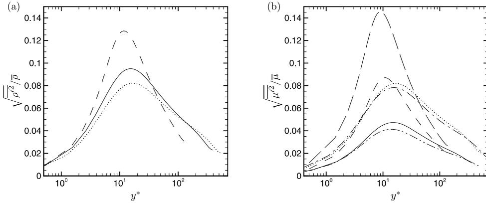
FIG. 2. Root mean square of (a) density fluctuations  $\sqrt{\rho'^2}/\bar{\rho}$ , (b) viscosity fluctuations  $\sqrt{\mu'^2}/\bar{\mu}$ . Lines are the same as in Figure 1.
