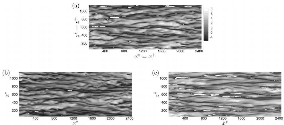
FIG. 16. Instantaneous stream-wise velocity fluctuations  $\sqrt{\rho u''}/\sqrt{\tau_w}$  in  $x^*-z^*$  plane at  $y^* \approx 15$ . Contour for  $\sqrt{\rho u''}/\sqrt{\tau_w} < -5.5$  are cut-off (seen as white). (a) Case CP395, (b) case LL, (c) case  $SRe_{\tau GL}^*$ .
