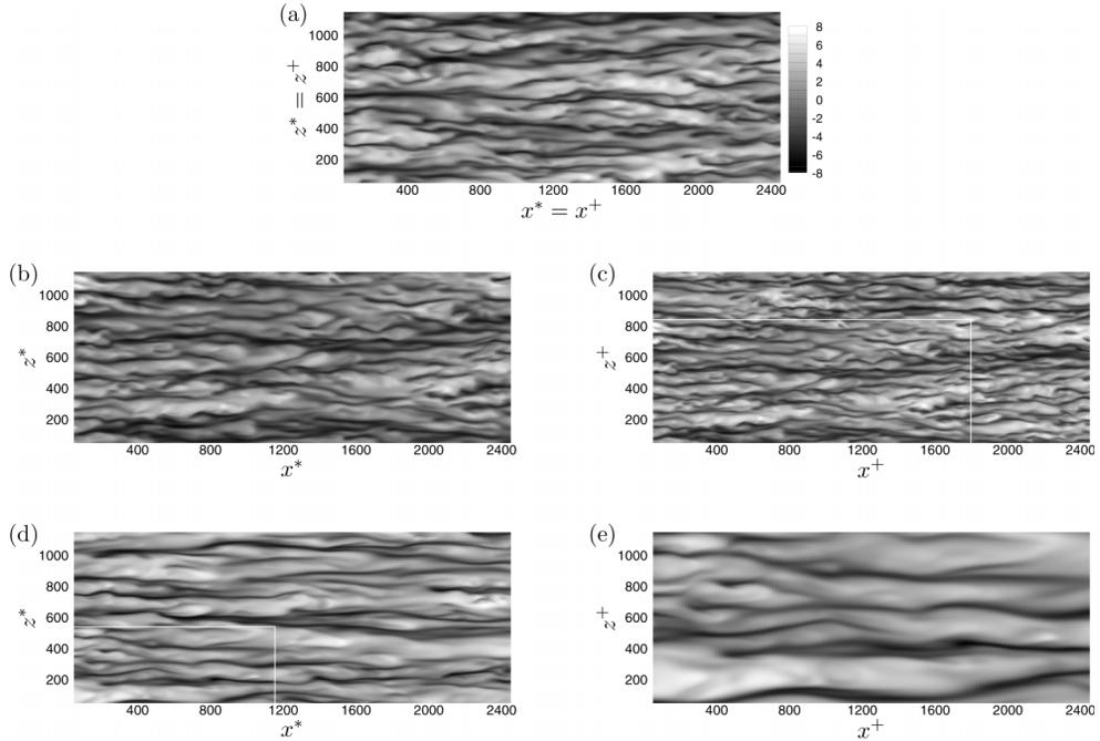
FIG. 15. Instantaneous stream-wise velocity fluctuations  $\sqrt{\rho u''}/\sqrt{\tau_w}$  in an  $x-z$  plane at  $y^* \approx 15$ . (a) Case CP395, (b) case LL using  $x^*-z^*$  co-ordinates, (c) case LL using  $x^+-z^+$  co-ordinates, (d) case  $SRe_{\tau GL}^*$  using  $x^*-z^*$  co-ordinates, and (e) case  $SRe_{\tau GL}^*$  using  $x^+-z^+$  co-ordinates. The white box in (c) corresponds to (b) and box in (d) corresponds to (e).
