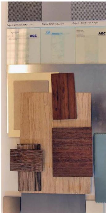
Figure 46 Base pallet - Natural and neutral materials are used for the base of the building are used. Such as metal, clear/translucent glass complemented by a wood finish (source: Ector hoogstad Architecten, 2015)
