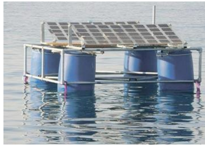
Figure 1.8: Floating PV Array [10].
