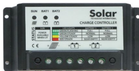
Figure 1.4: Charge controller for PV systems [4]
