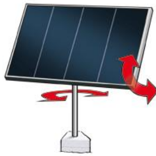
Figure 5.19: Azimuth-Tilting tracking system [9].
