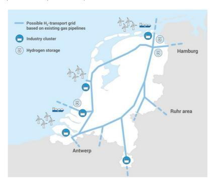
Figure 1: National Hydrogen Backbone (Gasunie, 2022)
