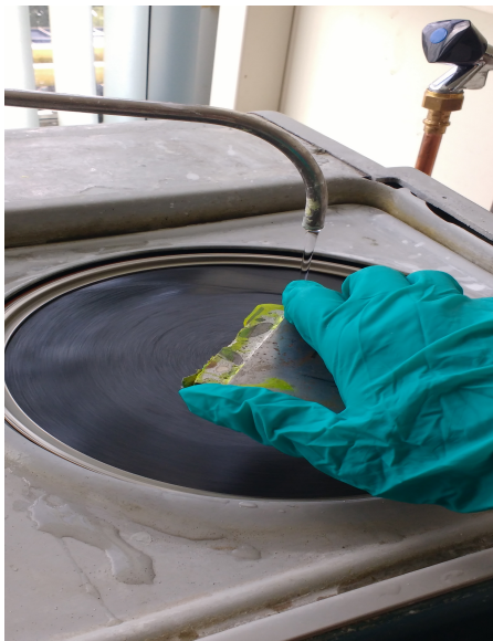
(c) Grinding on a lap table using SiC paper
