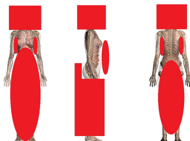
Figure A.1: Excluded material zones for exoskeleton according to ergonomic assumptions and working activities
