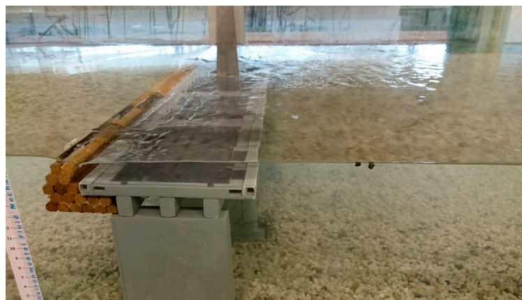
Figure 4. Laboratory setup, including debris damming on the upstream face of decks. The far deck is outfitted with the load cell, while the other two decks are free standing.
