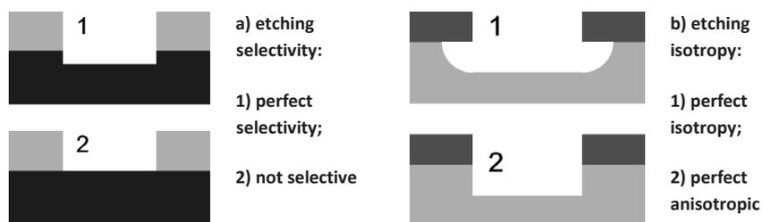
Figure 4 - Etching selectivity and isotropy
