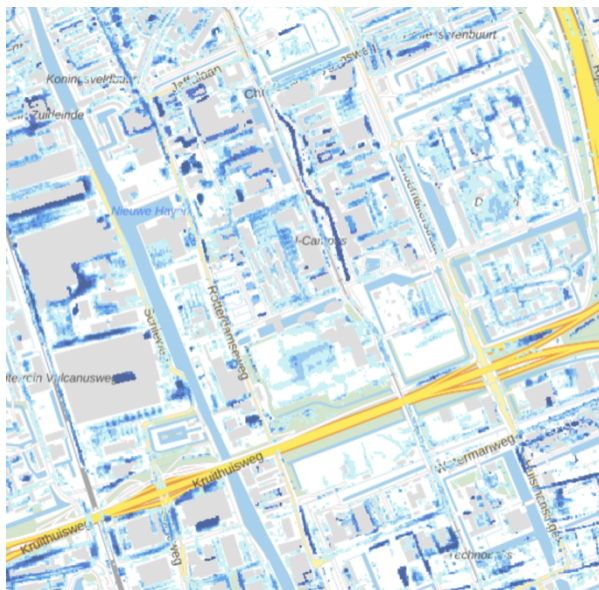
Figure 4-8: TUD Campus. Water depth rainfall 70 mm/ 2 hours (Stichting Climate Adaptation Services, n.d.)
