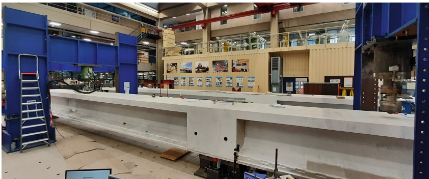
Fig. 3. Precast continuous girder in the lab (Left: Main girder Right: Cant. Beam)
