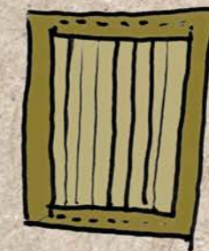
Reed clamped in frame
