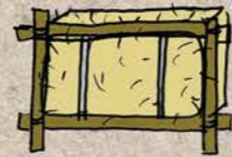
Miscanthus bailed on substructure
