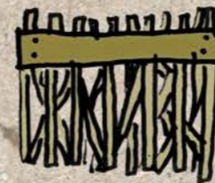
Reed clamped by wooden slat
