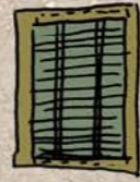
Willow withies weaved on frame
