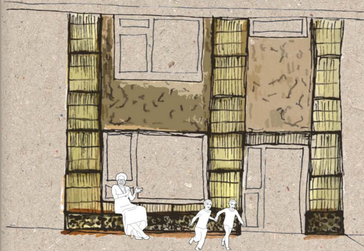
'Combined thatched and paneled reed'
