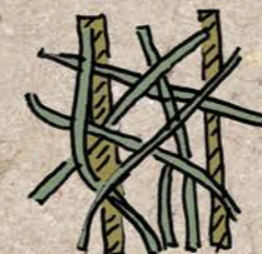
Willow withies randomly nailed on substructure
