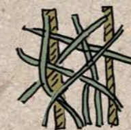
Willow withies randomly nailed on substructure
