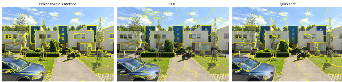
Figure 4.1: Segmentation algorithm comparison: Felzenszwalb's (scale=1200, sigma = 0.5, min size = 50), SLIC (segments = 50, compactnes=10), Quickshift (Kernel size = 12)
