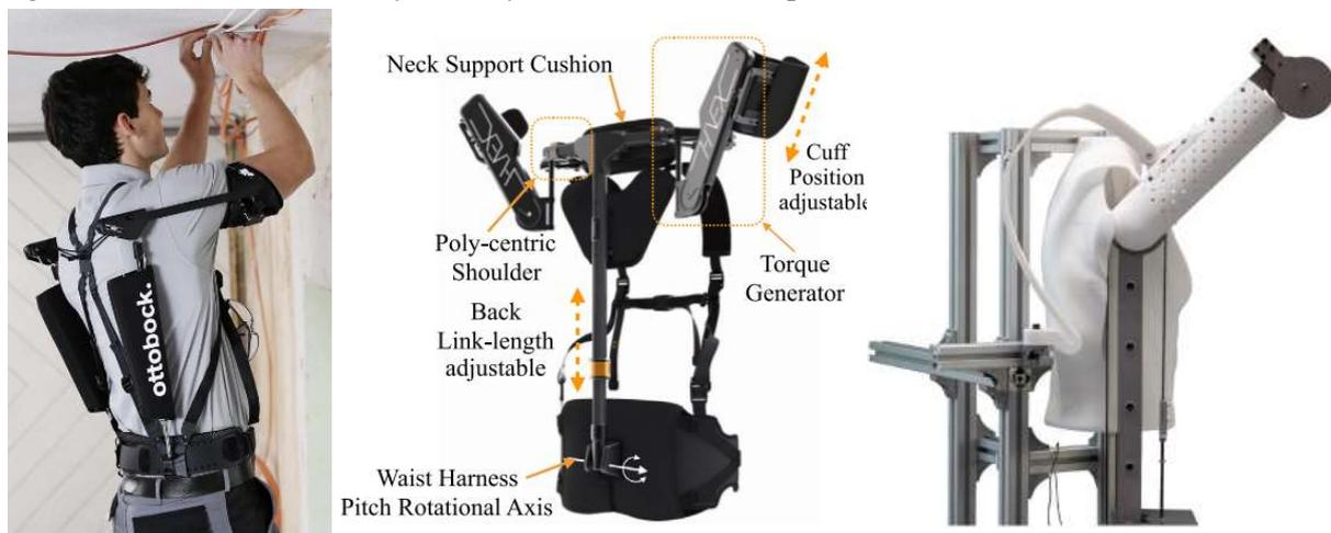
Figure 1.1. Left-Paexo Shoulder[2], middle-H-VEX[5], right-Tschiersky's compliant shoulder exoskeleton[4]
