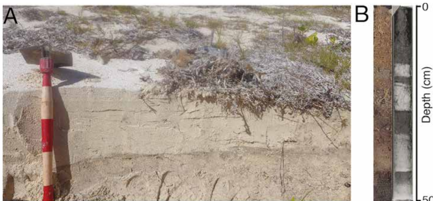
Figure 1: (A) Hurricane Irma (2017) sediments deposited on top of beach sand on the island of Anegada, British Virgin Islands. The deposit represents an important modern analogue for interpreting a series of paleo-storm and tsunami deposits preserved within coastal ponds on the island. (B) Overwash deposits (sands and silts) from historical storms (photograph and X-ray view) recorded within saltmarsh peat at Succotash Marsh, Rhode Island, USA. Cores were taken in close proximity to those in Donnelly et al. (2001).
