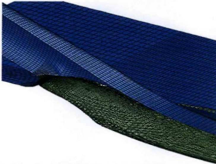
Figure 7.6 Example of triangular surface mesh of streamtube surface (in green). Rectangular cells represent solid wall cells of waterjet inlet in blue.
