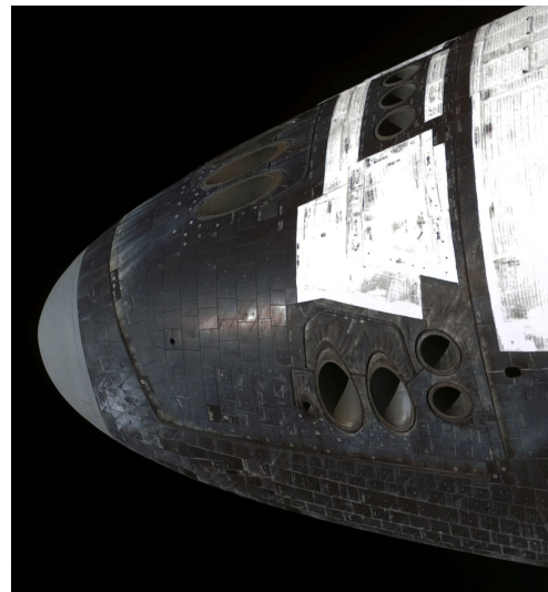
(b) Front port thruster assembly of the Space Shuttle. Copyright-free.
