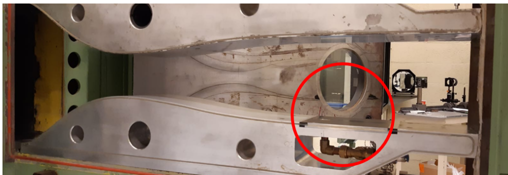
Figure 3.4: Photograph showing the Mach-2 converging-diverging nozzle with the position of the jet nozzle highlighted in red.
