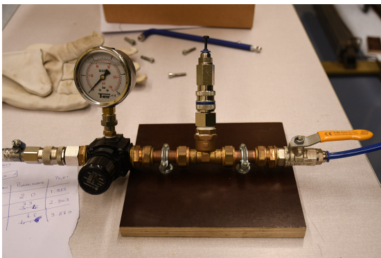
(a) Upstream assembly (pressure regulator, PIV seeding line and safety shut-off valve).
