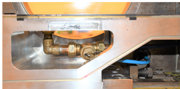
(b) Downstream assembly (thermocouple and Pitot tube and sonic nozzle).
