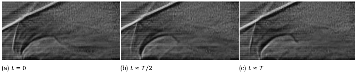
Figure 5.23: Shadowgraph images of the sonic jet at J = 2 at high frame rate, focused on the barrel shock.
