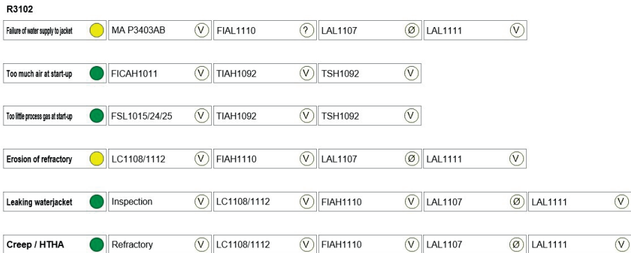
Fig. 5.9, screenshot of the process safety dashboard of the post reformer
