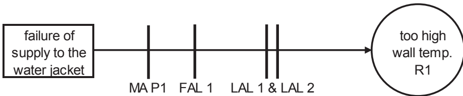
Fig. 5.6, scenario 'too high wall temperature R1' by failure of the water jacket cooling
