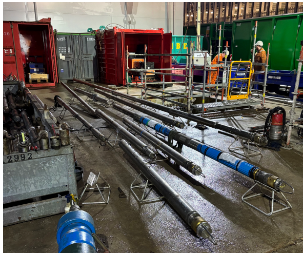
Figure 2.3: BakerHughes micro-frac wireline tool, later to be used for performing a micro-frac test at the DEL-GT-02 well in Delft. Note the blue protection, which denote the packers on the tool.
